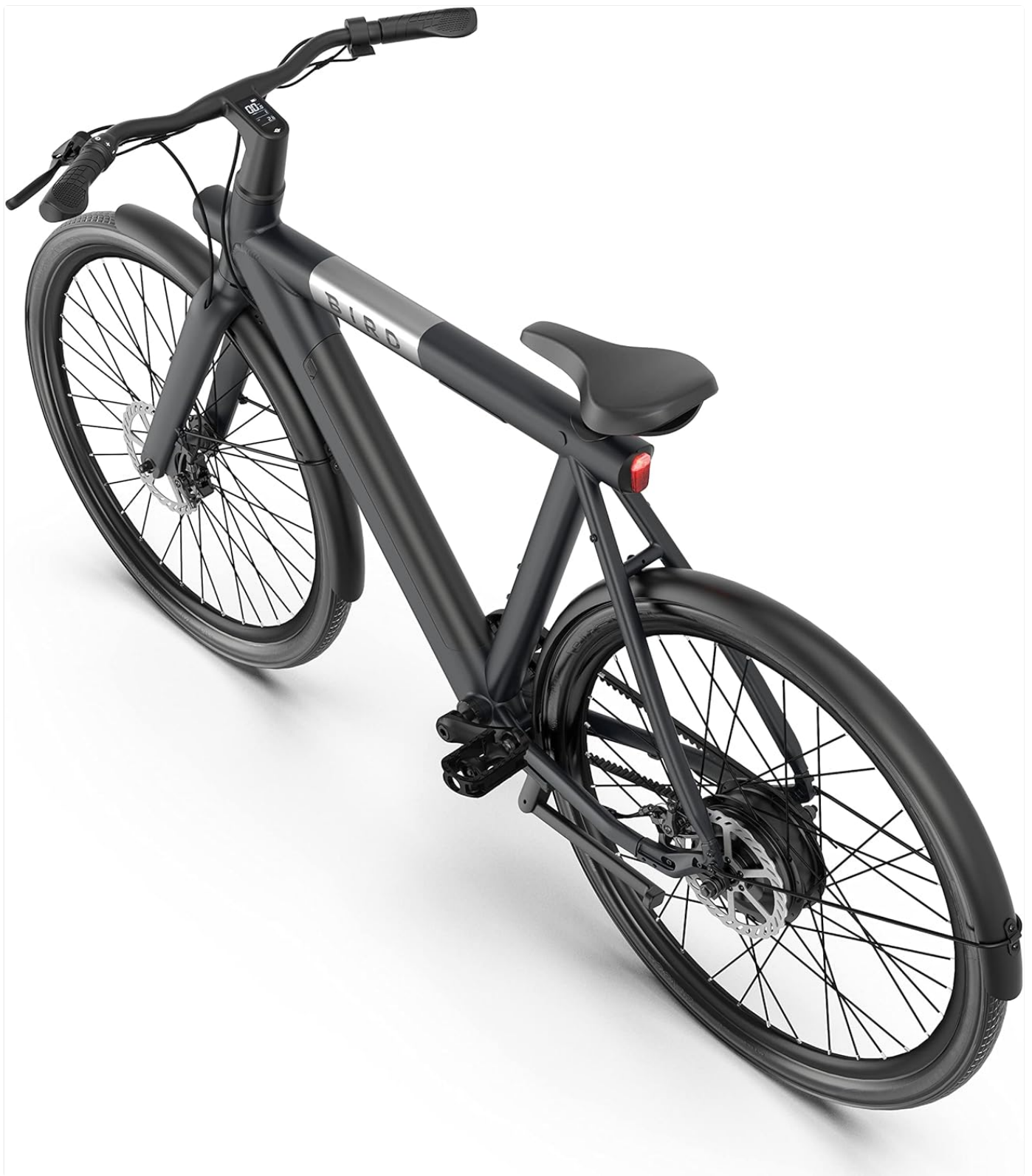
Image: Rear-angle view of the BirdBike A-Frame eBike, showing the rear wheel, belt drive, and integrated taillight.
