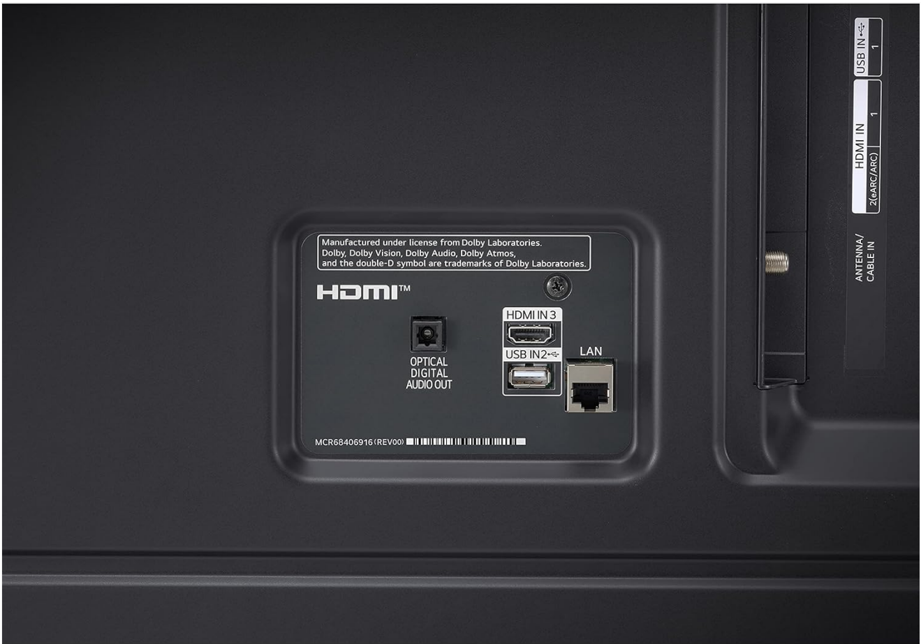
Image 1.2: Rear panel connections showing HDMI, USB, LAN, and Optical Digital Audio Out ports.
