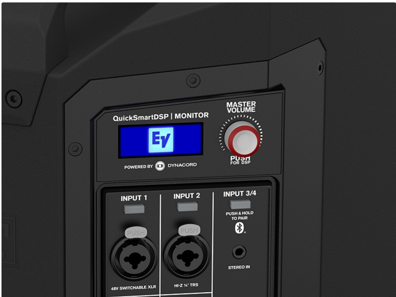
Figure 3.1: The QuickSmartDSP display and Master Volume knob for comprehensive control.
