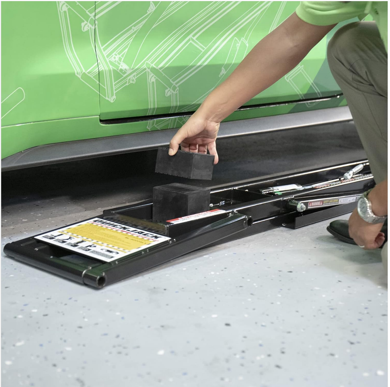
Figure 4.2: Placing the rubber lifting blocks onto the frames.
