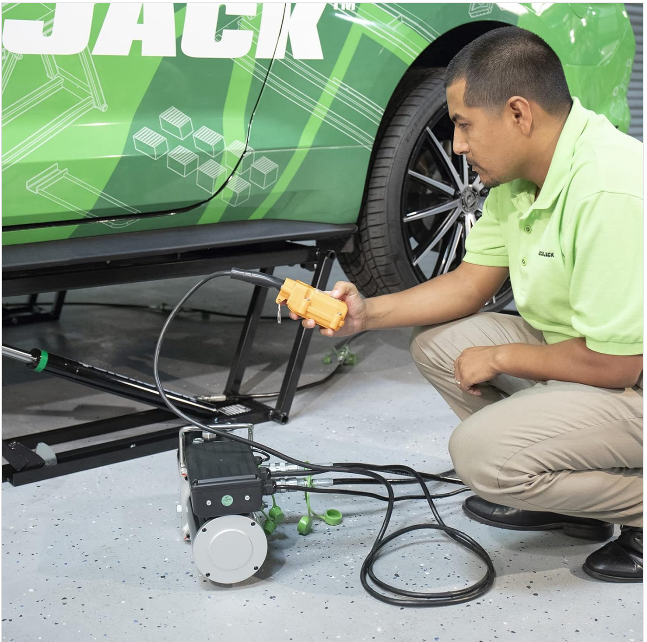
Figure 4.3: Connecting the quick-connect hydraulic hoses to the power unit.
