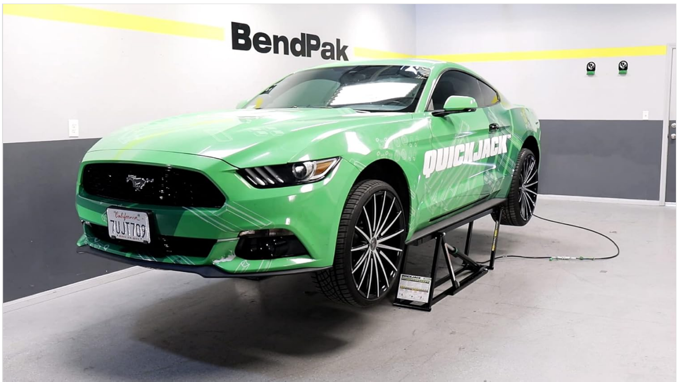
Figure 5.1: Vehicle positioned over the QuickJack frames, ready for lifting.
