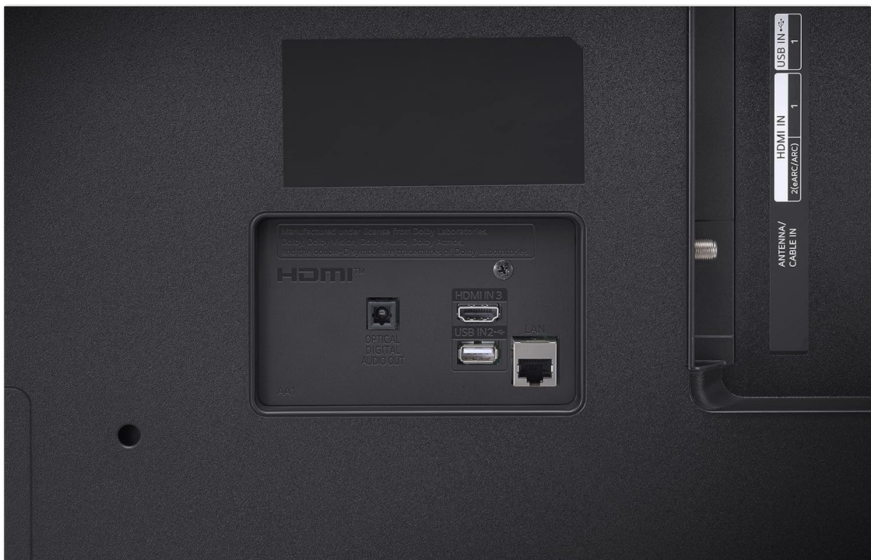
Image: A close-up of the LG 65UQ9000PUD TV's HDMI, USB, and LAN ports, showing their labels and arrangement.
