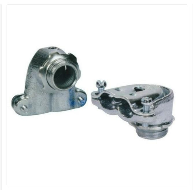
Image: Two Morris Products 15067 90 Degree Flex Duplex Box Connectors. These zinc die-cast connectors feature a 90-degree bend, designed for connecting two pieces of flexible metallic conduit or various types of sheathed cables to an electrical box.
