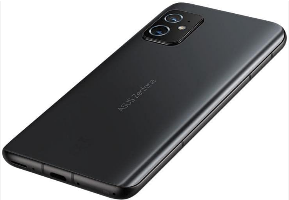
Figure 3.3: Angled view of the ASUS ZenFone 8, illustrating the placement of side buttons, USB-C port, and speaker grilles.
