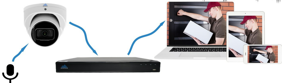
Figure 11: Diagram illustrating one-way audio transmission from the camera's built-in microphone to the NVR and remote devices.
