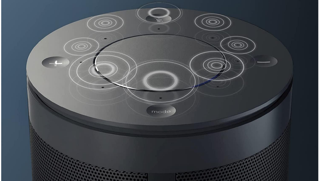
Image: Top view of the NexiGo Meeting 360, illustrating the eight omnidirectional microphones and touch controls for volume and mute.
