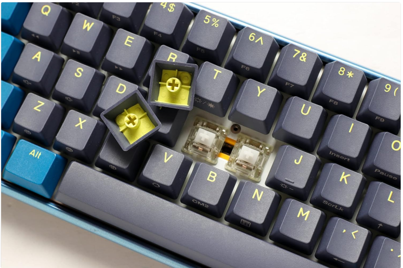
A close-up view demonstrating the hot-swappable nature of the switches, with a keycap and switch removed to reveal the socket.
