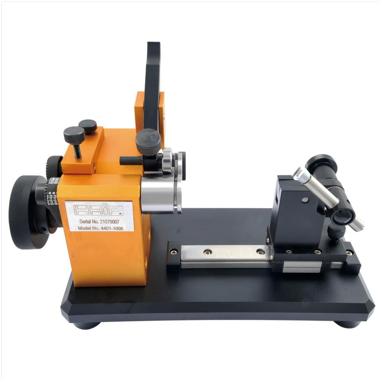
Figure 1: HHIP 4401-1006 Universal Single Indicator Concentricity Checker with a dial indicator.
