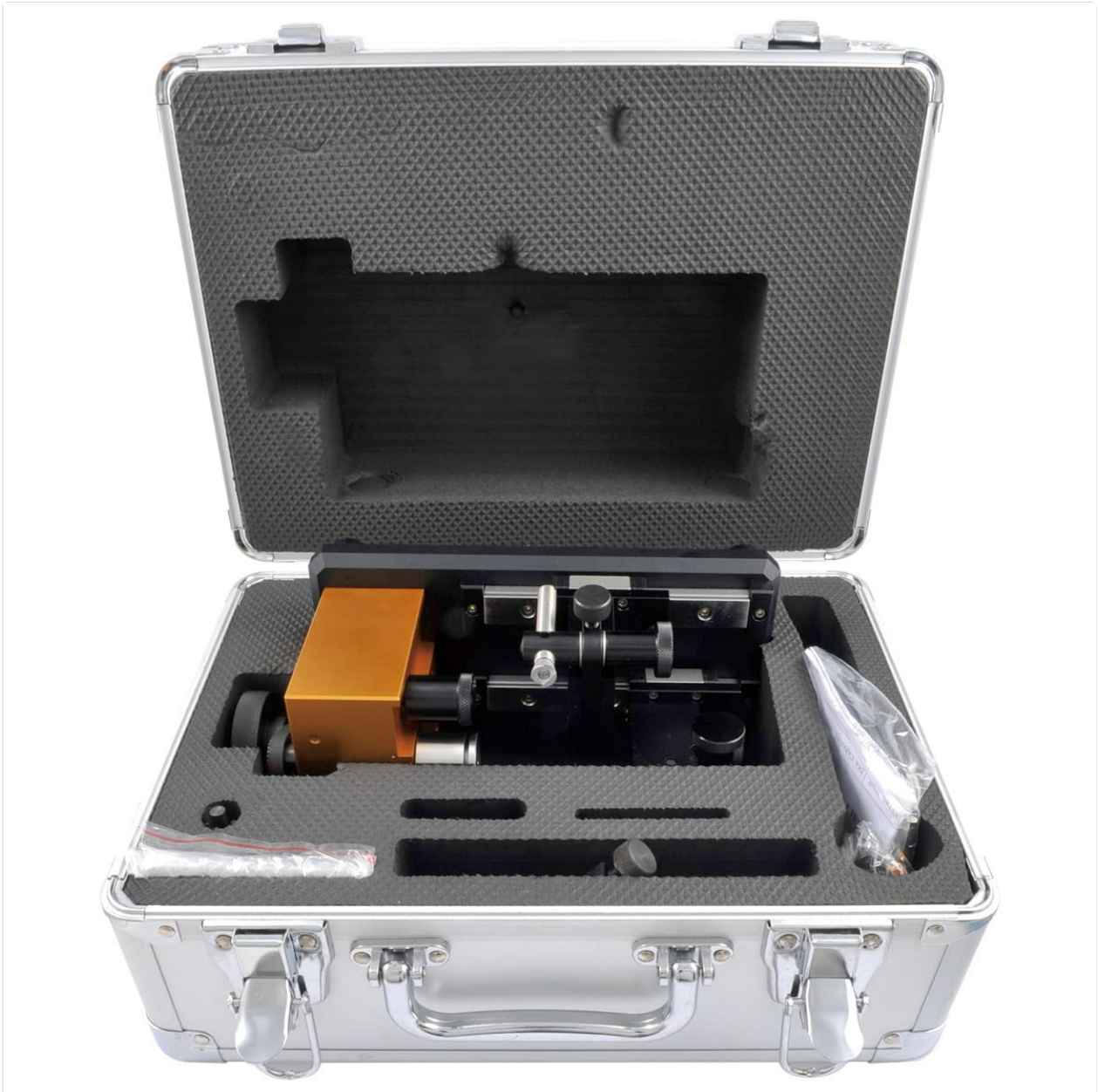
Figure 4: Concentricity checker stored in its protective case.
