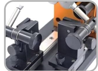
Figure 3: Detailed view of the concentricity checker with operational notes.
