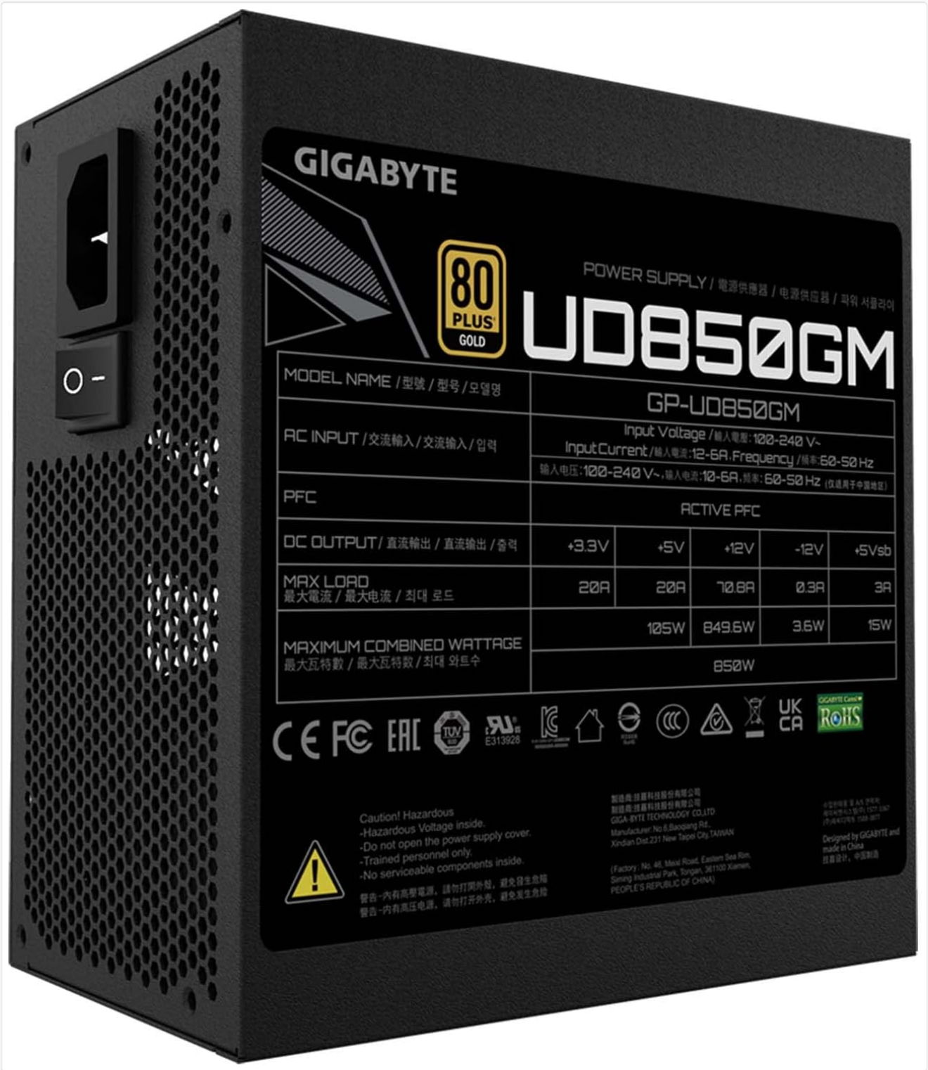
Image: Side view of the GIGABYTE GP-UD850GM power supply, clearly displaying the product specification label. This label
