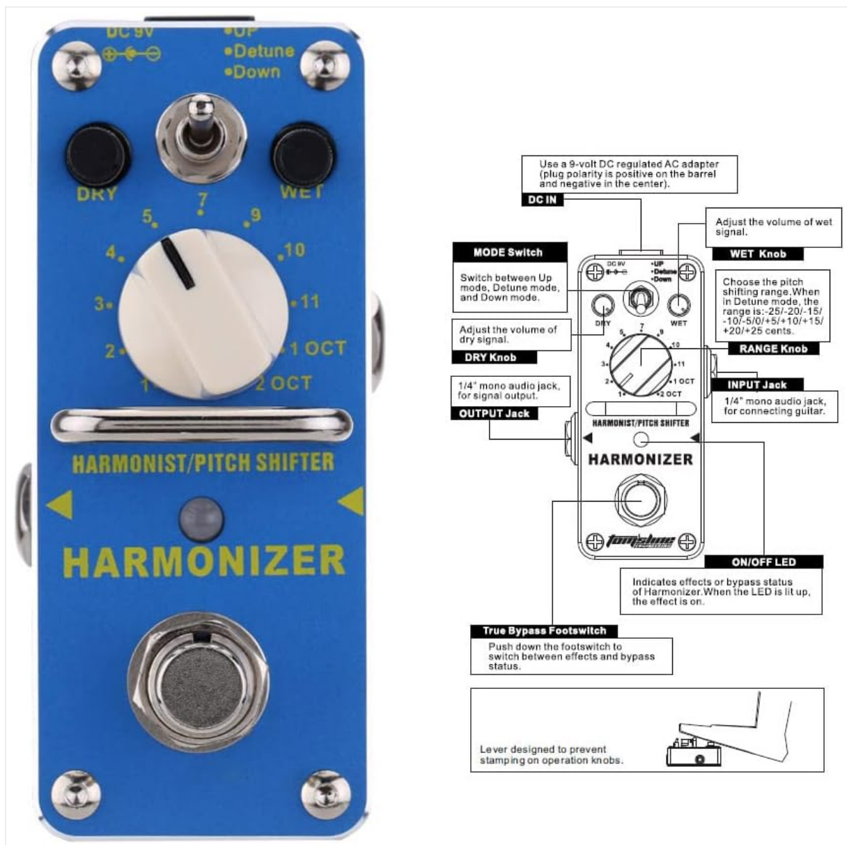
Figure 3.1: Diagram illustrating the input, output, DC power connections, and control layout of the AHAR-3 Harmonizer pedal.
