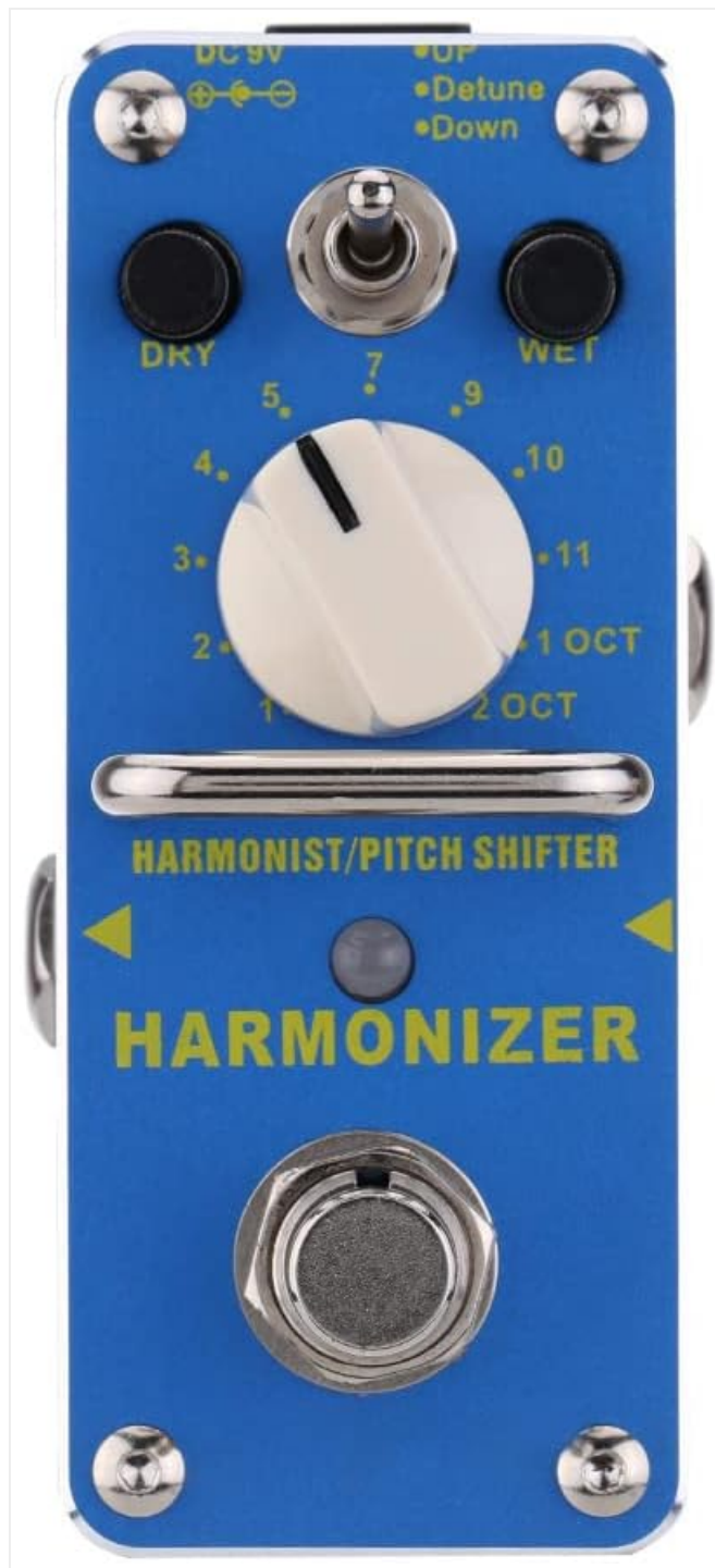
Figure 4.1: Close-up view of the AHAR-3 Harmonizer pedal's controls, including DRY, WET, and RANGE knobs, and the MODE switch.
