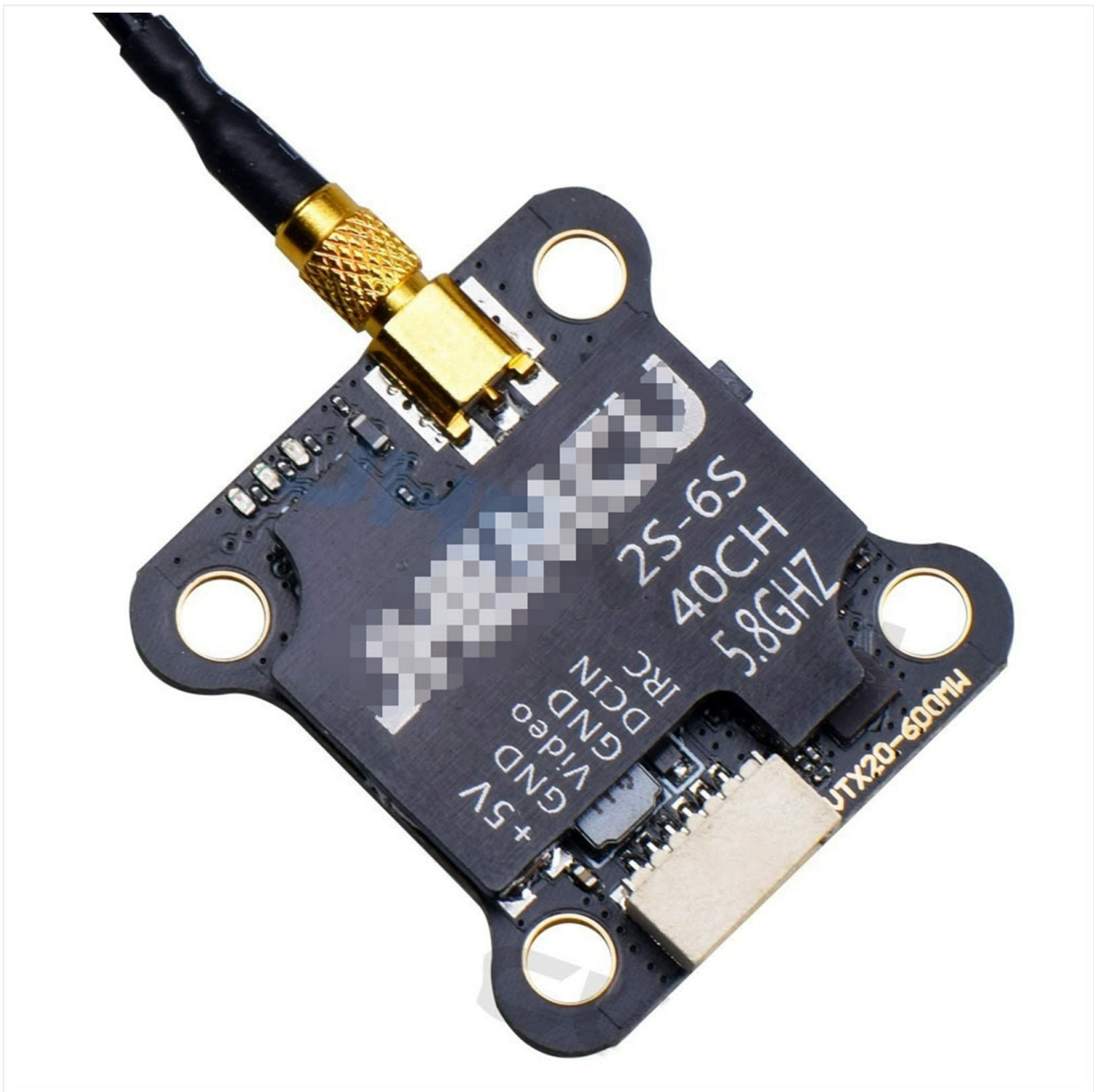
Image 1.1: JHEMCU VTX20-600 FPV Transmitter with included antenna and wiring harness.
