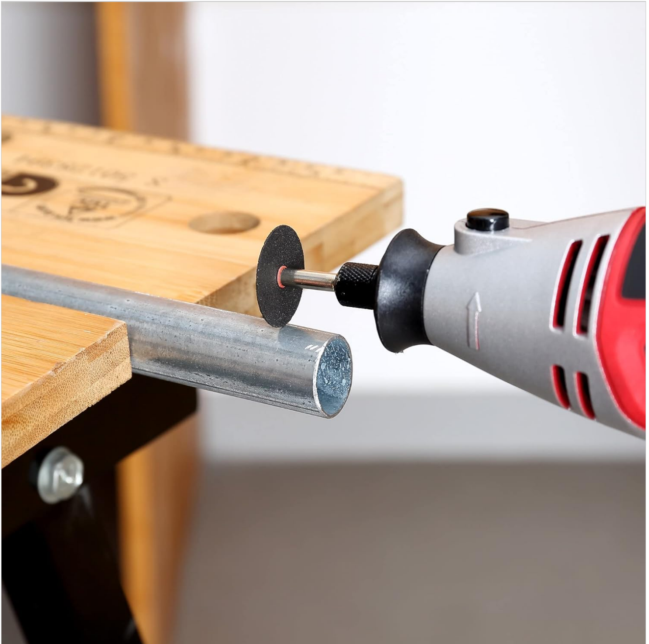
Image 5: Using a cut-off wheel to cut a metal pipe.
