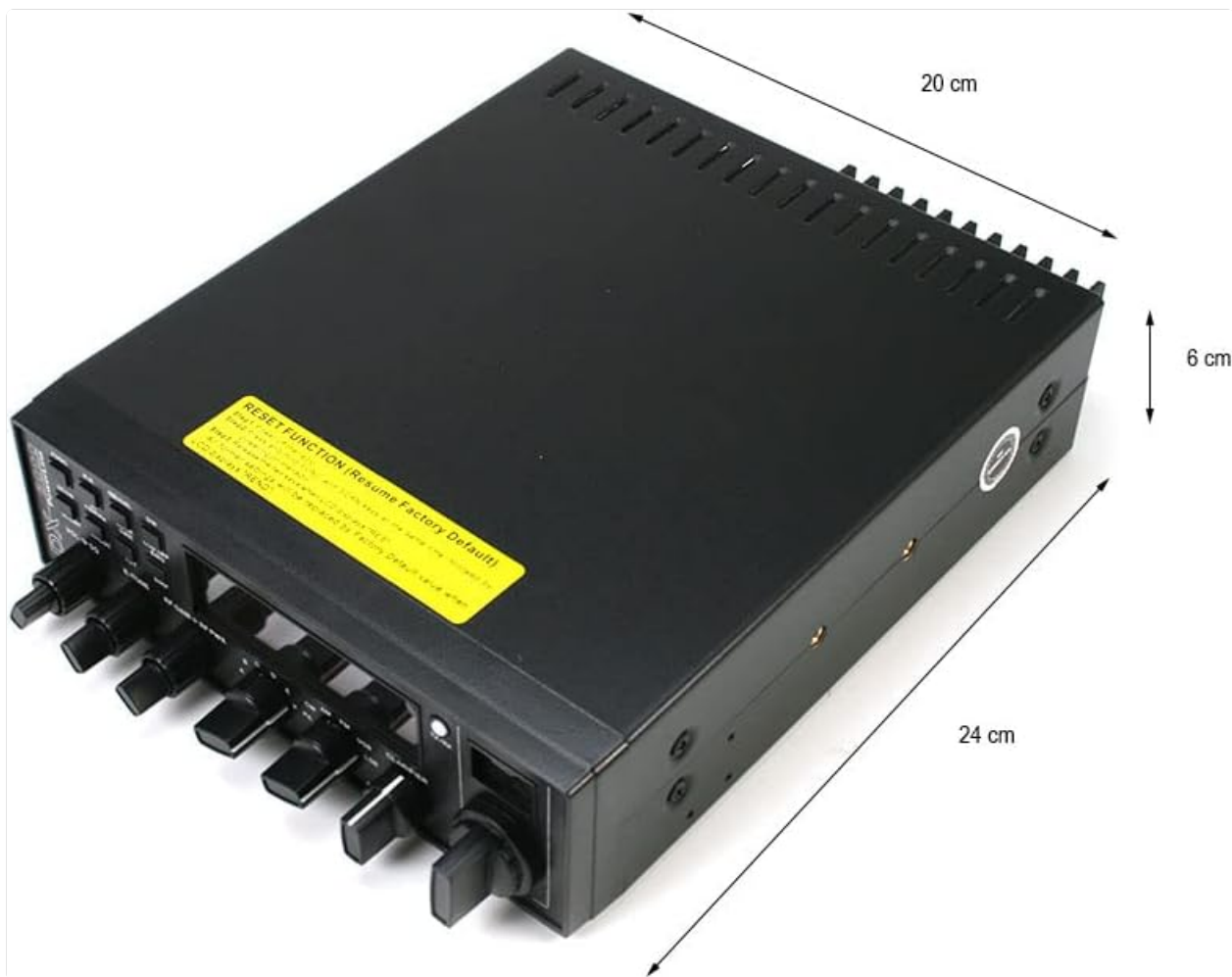
Figure 7.1: Diagram illustrating the physical dimensions of the K-PO DX 5000PLUS Transceiver, showing its length, width, and height in centimeters.
