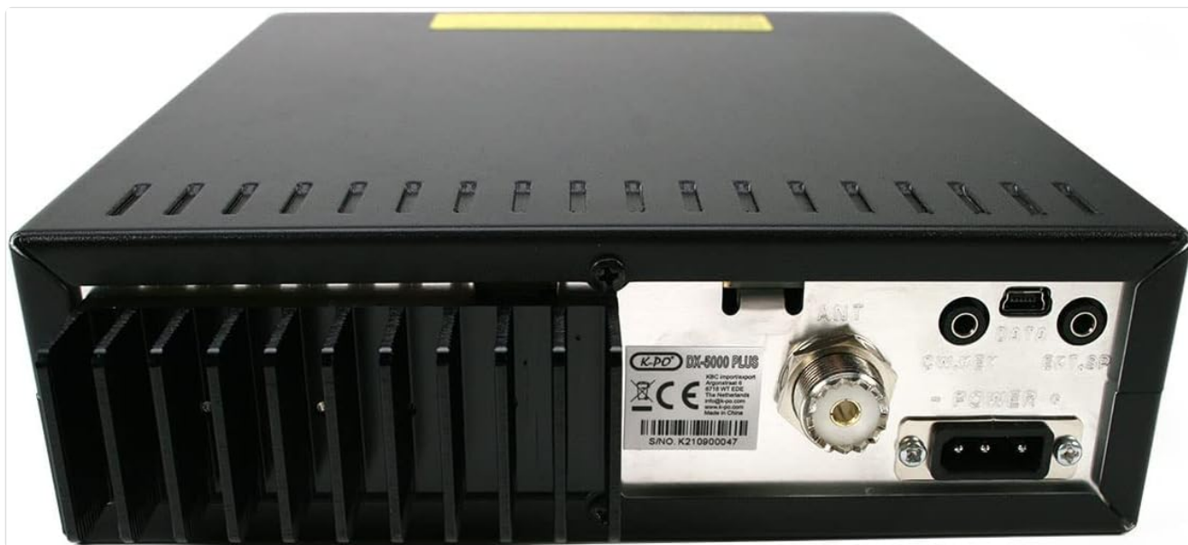
Figure 3.2: Rear panel of the K-PO DX 5000PLUS, showing antenna connector, power input, and data ports. This view is crucial for understanding how to connect the transceiver to external components.
