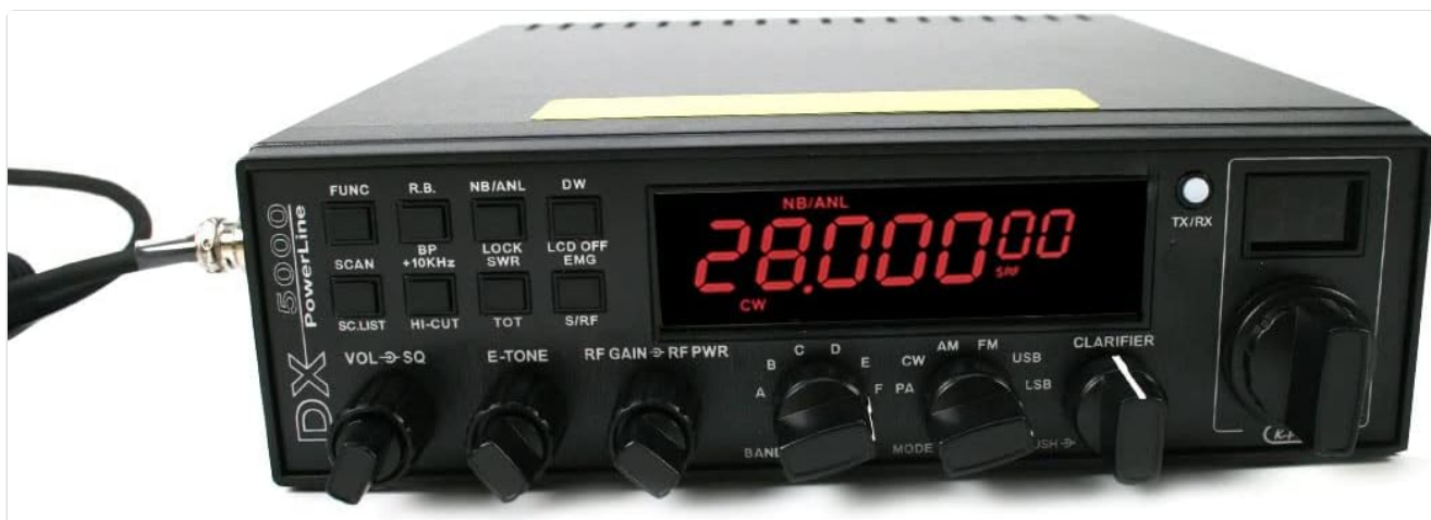
Figure 3.1: Close-up view of the K-PO DX 5000PLUS front panel, showing the display, buttons, and rotary controls for various functions like volume, squelch, RF gain, and mode selection.
