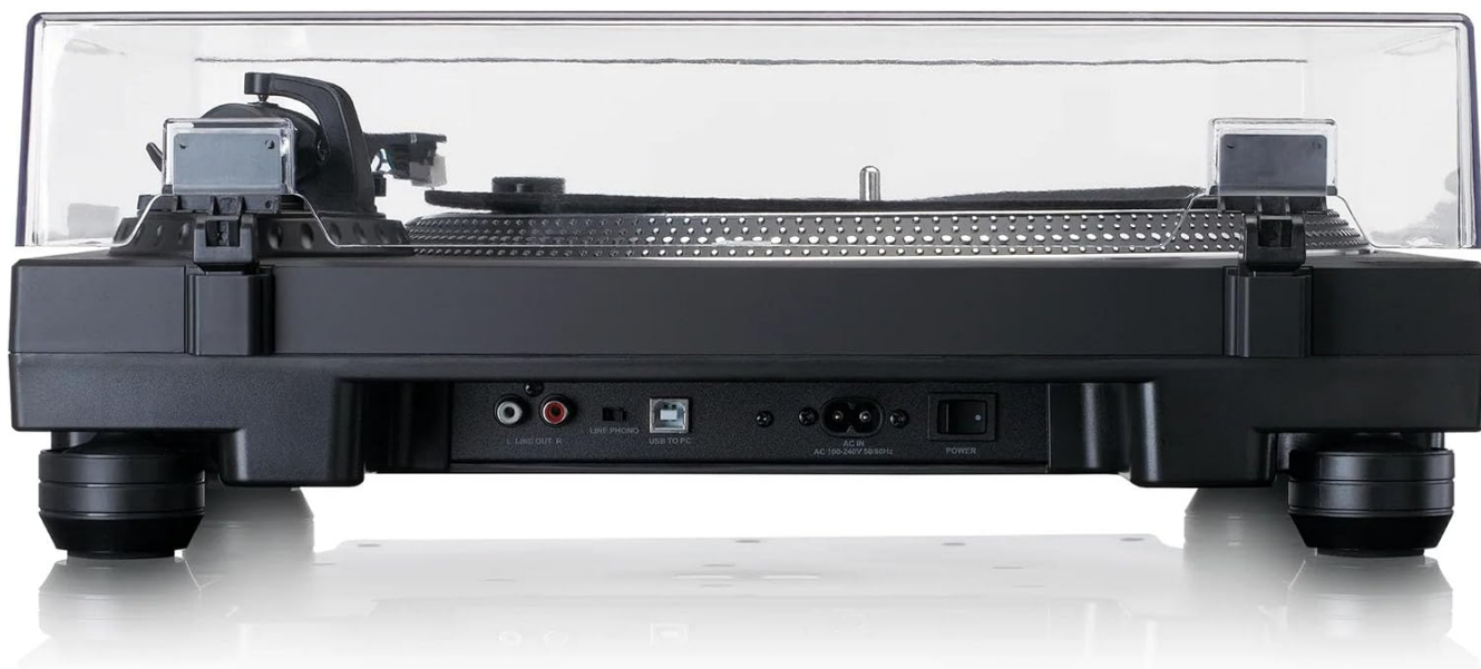
Figure 3: Rear view of the Lenco L-3818 turntable, displaying the connectivity ports. From left to right, these include the RCA Line-Out (L/R), a switch for Line/Phono output, a USB port for PC connection, the AC power input, and the main power switch.
