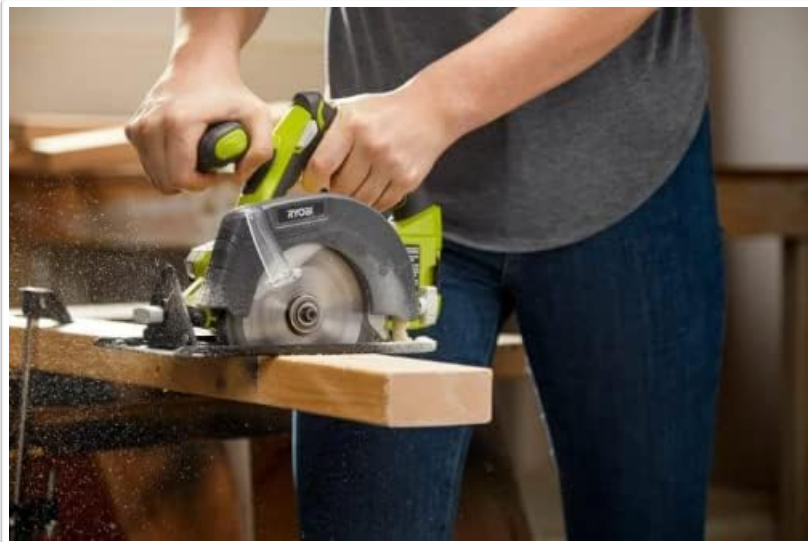
Figure 5: An individual demonstrating proper technique for cutting wood with the circular saw.
