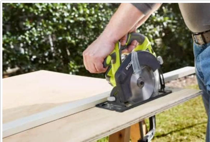
Figure 6: Detailed view of the saw in operation, cutting through a wooden board.
