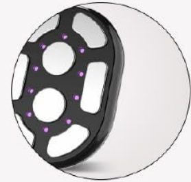
Image 4.2: The device indicating different operational modes via colored LED lights.
