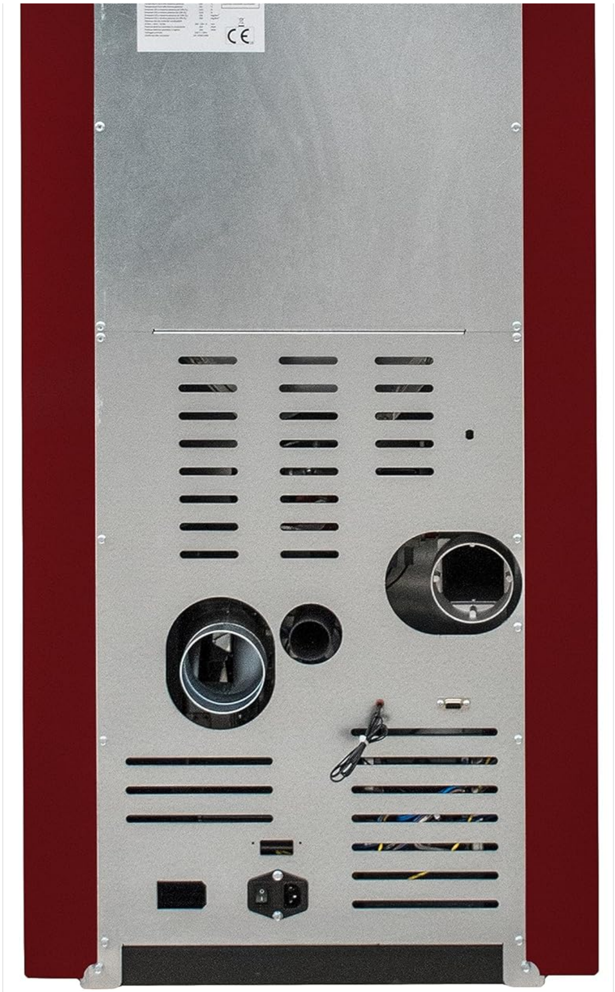
Figure 3.3: Rear Connections. This image shows the back of the stove, detailing the exhaust outlet (80mm diameter) and electrical
