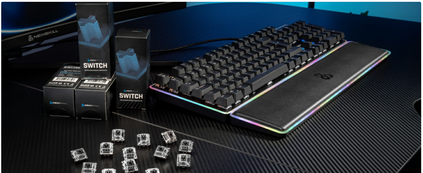
Image: The Newskill Gungnyr Pro Ivory keyboard on a desk, surrounded by individual Gateron switches and their packaging, illustrating the hot-swappable feature.
