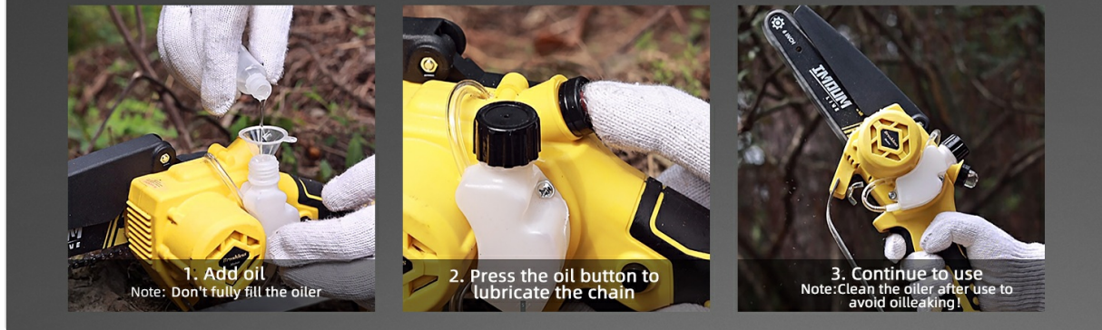
Image: Steps for adding oil to the auto-lubrication system.
