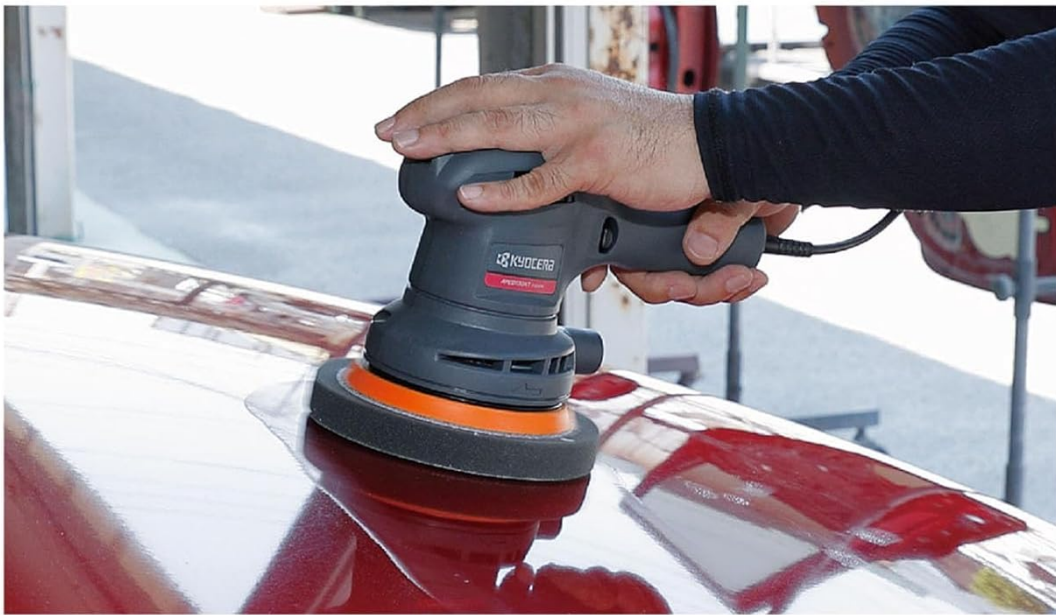
Figure 6.2: The polisher's ergonomic design facilitates comfortable two-handed or one-handed operation.
