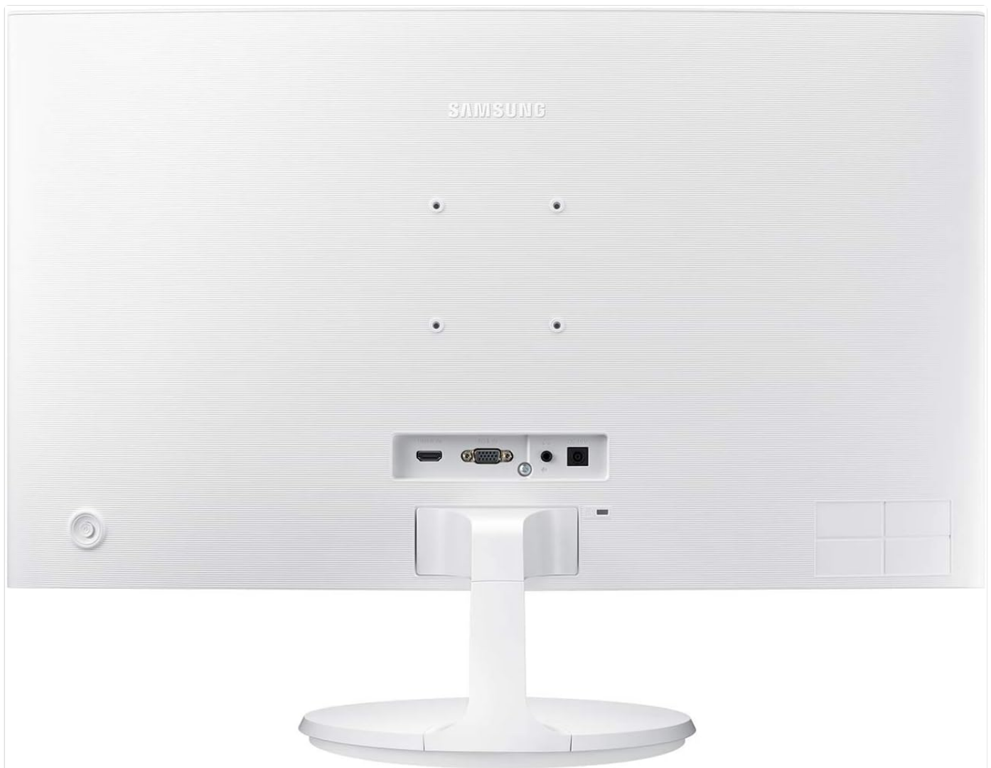
Image: Detailed view of the monitor's rear input panel, showing HDMI IN, D-Sub, Headphone Jack, and DC IN ports.
