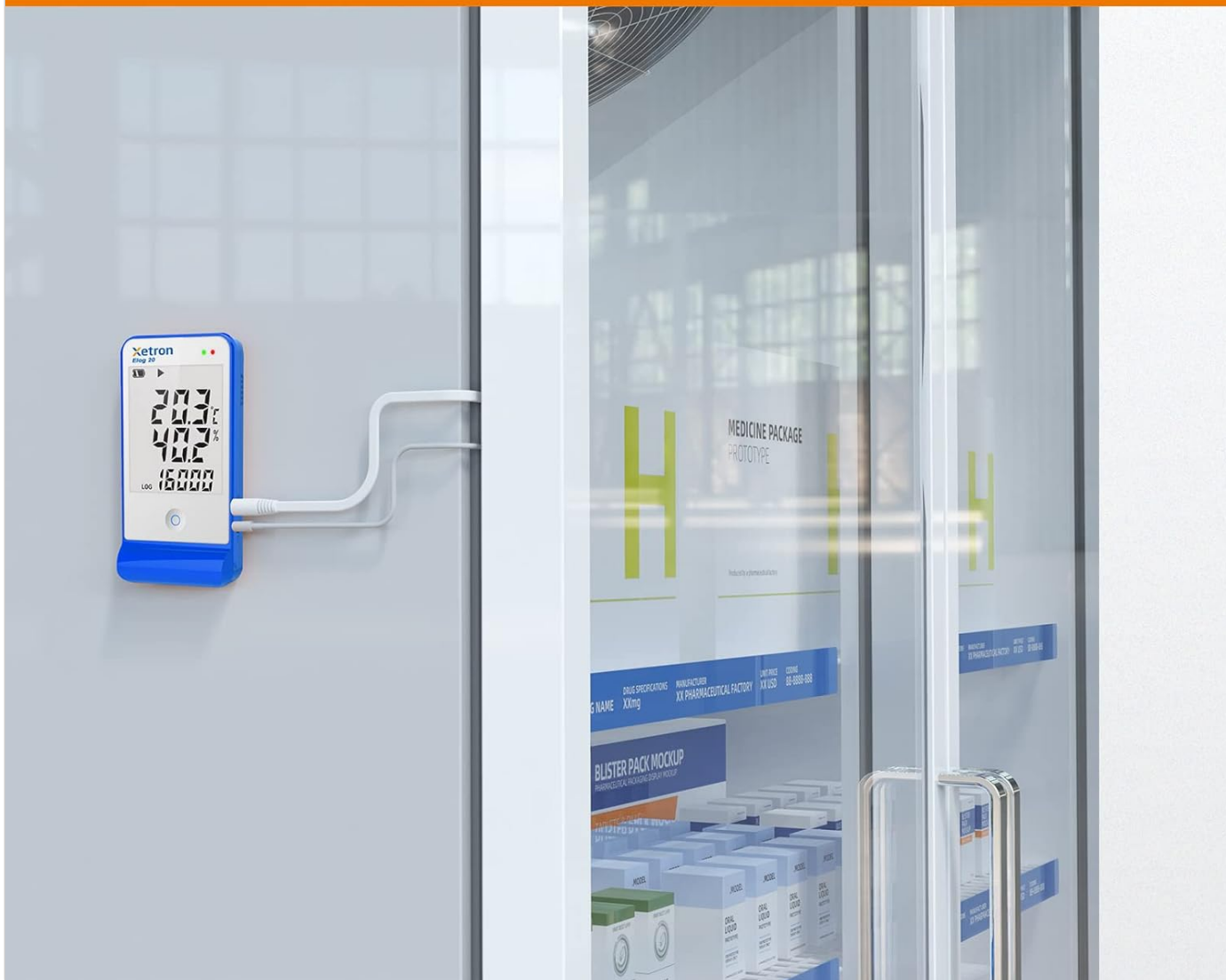
Image: The Xetron Elog20 data logger demonstrating its built-in magnets for easy attachment to a refrigerator door, illustrating one of its three fixing methods.
