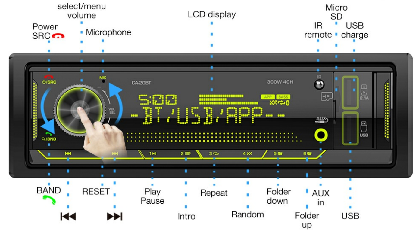
Image: Detailed diagram of the receiver's front panel, highlighting the power/source button, microphone, volume/select knob, LCD display, IR remote sensor, 2.1A USB charging port, standard USB port, AUX input, and various function buttons for playback control and band selection.
