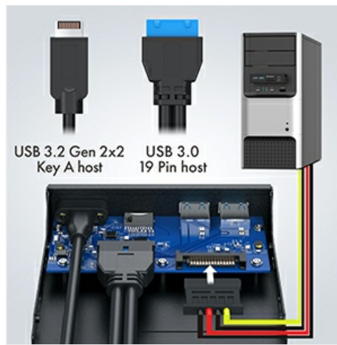
Image 4.4: Diagram showing the connection of the USB 3.2 Gen 2 Key A host and USB 3.0 19 Pin host cables to the motherboard, along with the SATA power connection.
