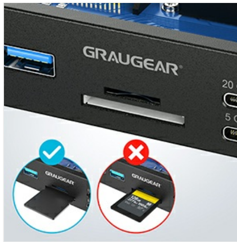
Image 5.3: Guide for correct SD card insertion (label down).
