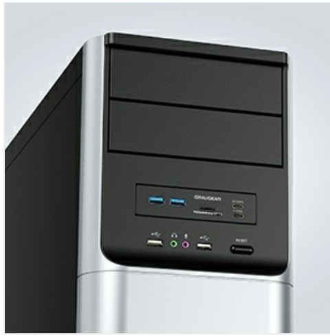
Image 4.2: The front panel hub installed in a 3.5-inch bay of a desktop computer.
