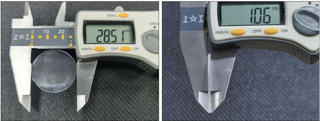
1. Lay the glass len flat and measure the diameter.
