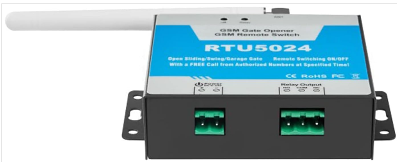
Figure 2.2: Angled view of the RTU5024, highlighting the power input terminals (DC 9-24V) and the relay output terminals (NO, COM, NC) for connecting to external devices like gate motors or door locks.
