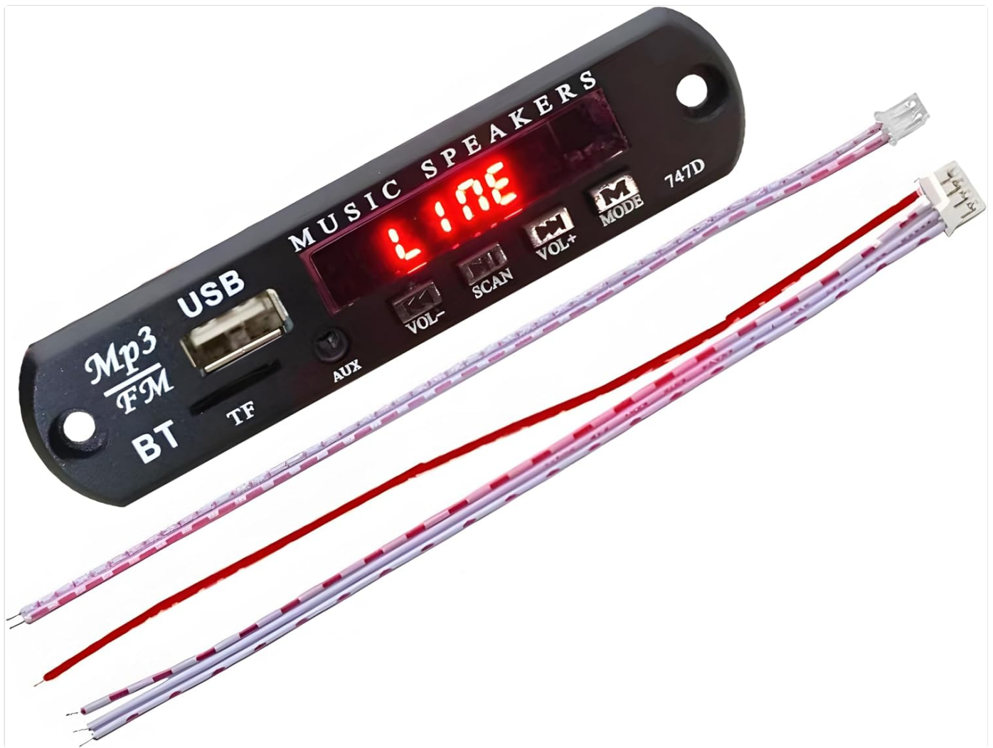
The decoder board displaying 'LINE' mode, indicating AUX input is active.
