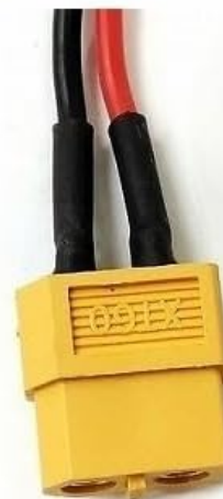
Image: The Li-ion 7.4V 1800mAh battery with its XT60 connector, ready for installation into the tank.
