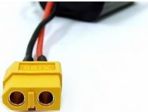
Image: The Li-ion 7.4V 1800mAh battery with its XT60 connector, ready for installation into the tank.
