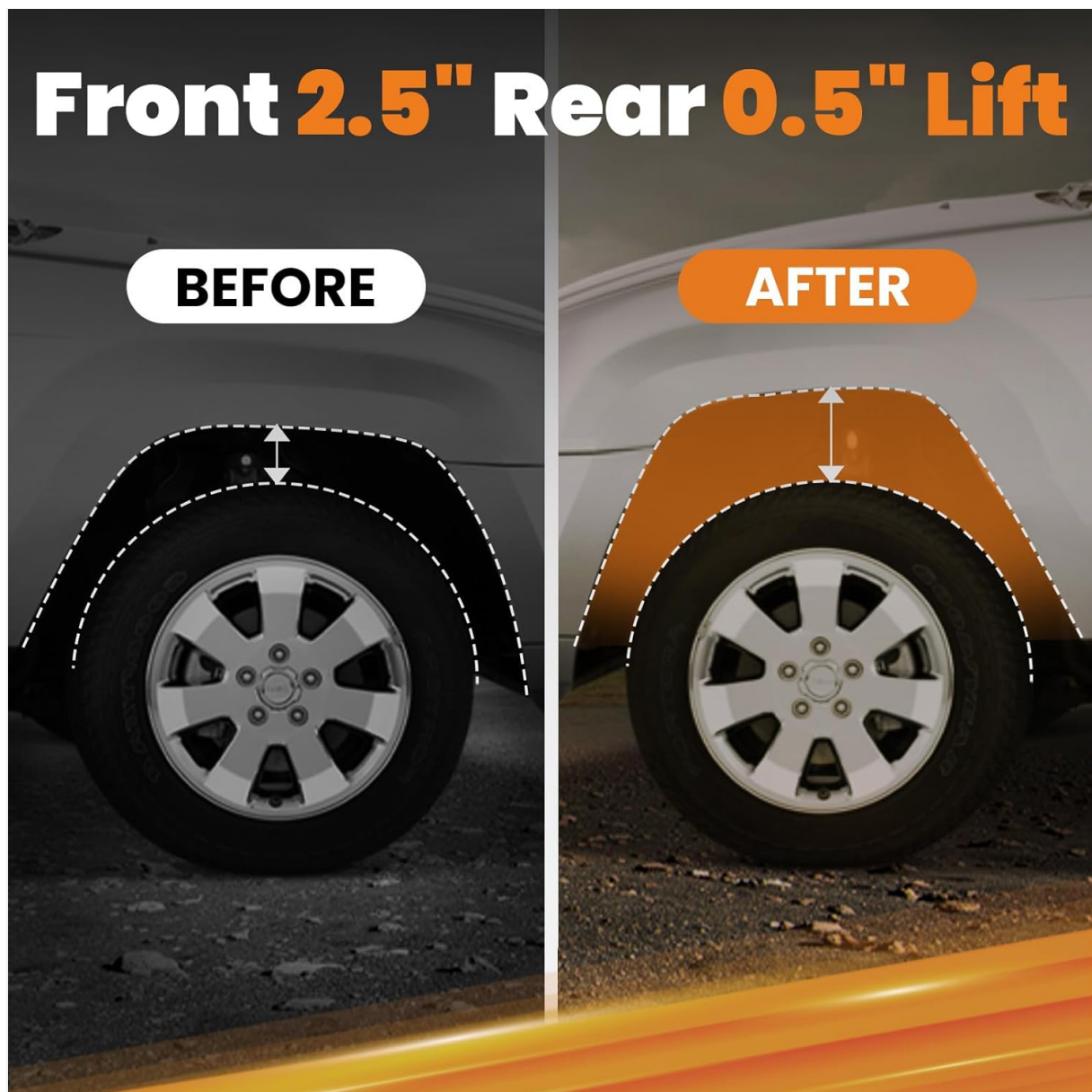
Figure 6: Visual comparison of a Jeep Grand Cherokee WK2 before and after the installation of the 2.5" front and 0.5" rear lift kit, demonstrating the increased ground clearance.
