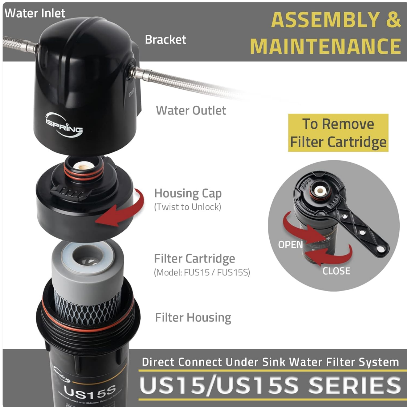
Figure 1: Assembly and Maintenance Diagram for iSpring US15/US15S Series
