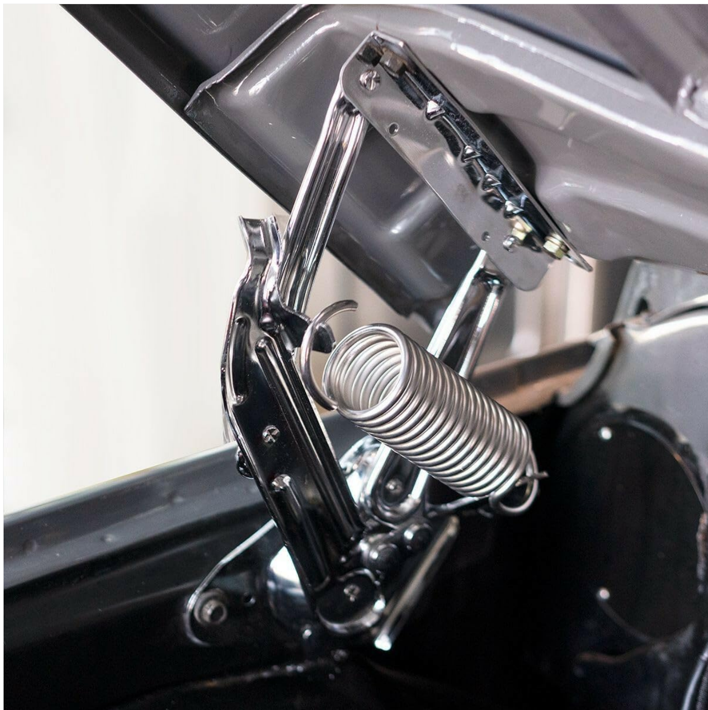
Image: The chrome hood hinge shown installed on a vehicle, with a spring attached, demonstrating its functional position.
