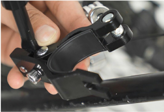
7. Mounting telescopic rod quick release head
