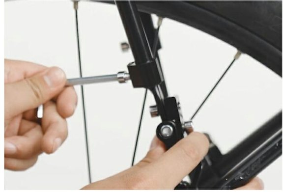
6. Adjust the the telescopic rods
