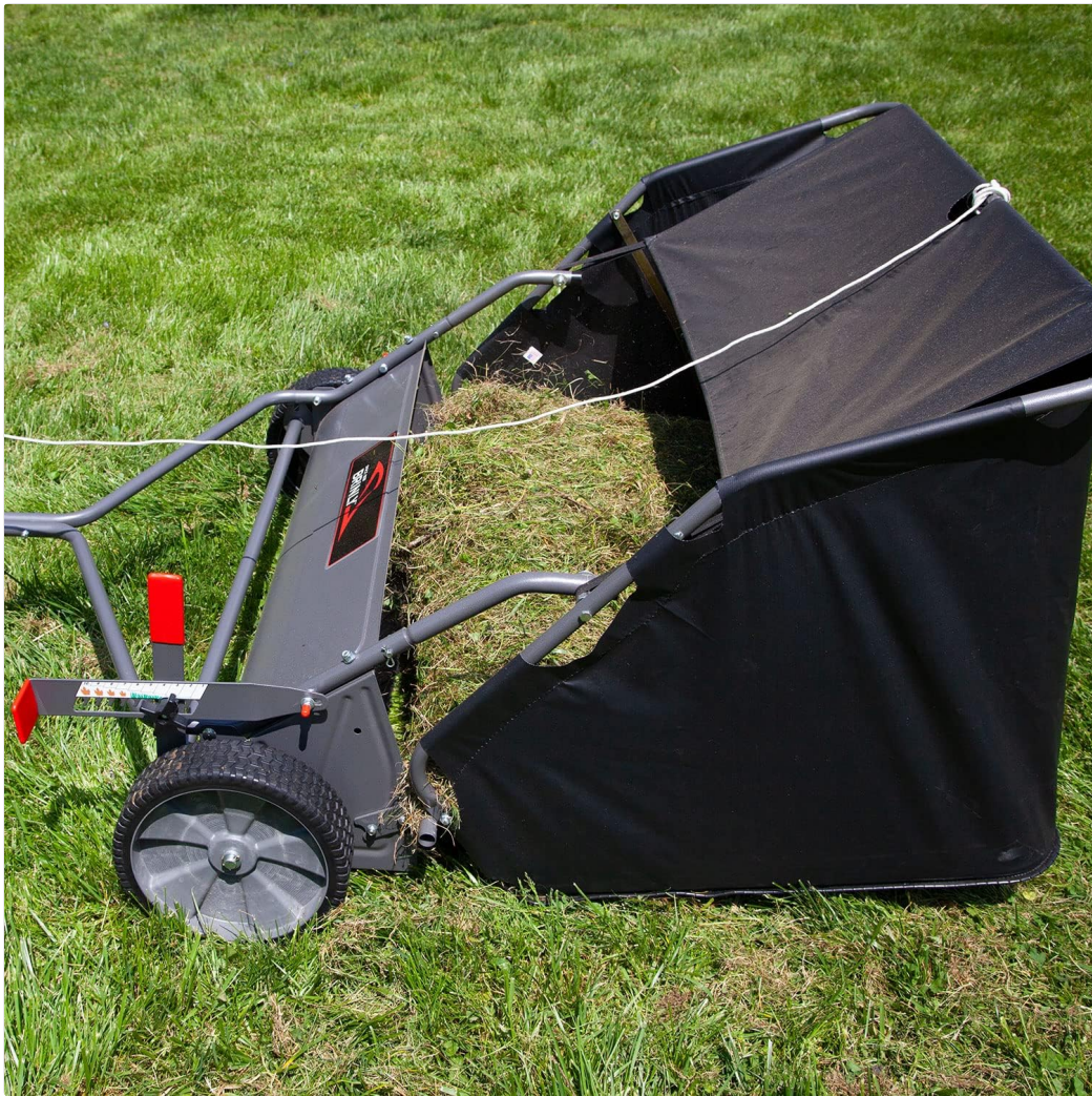
Figure 4.2: Close-up of the sweeper collecting grass clippings into the hamper.
