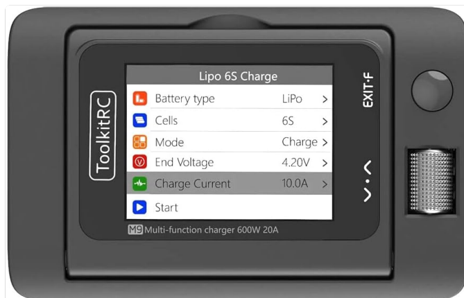
Image 3: A close-up of the ToolkitRC M9's color display, showing the menu for setting up a LiPo 6S battery charge, including battery type, cell count, mode, end voltage, and charge current.
