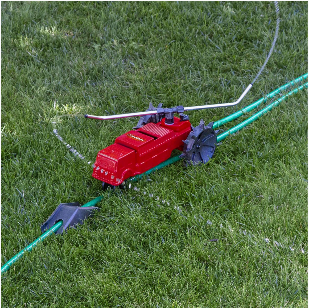
Image 4.2: The sprinkler positioned on the hose path, with the stop ramp at the end to trigger automatic shut-off.
