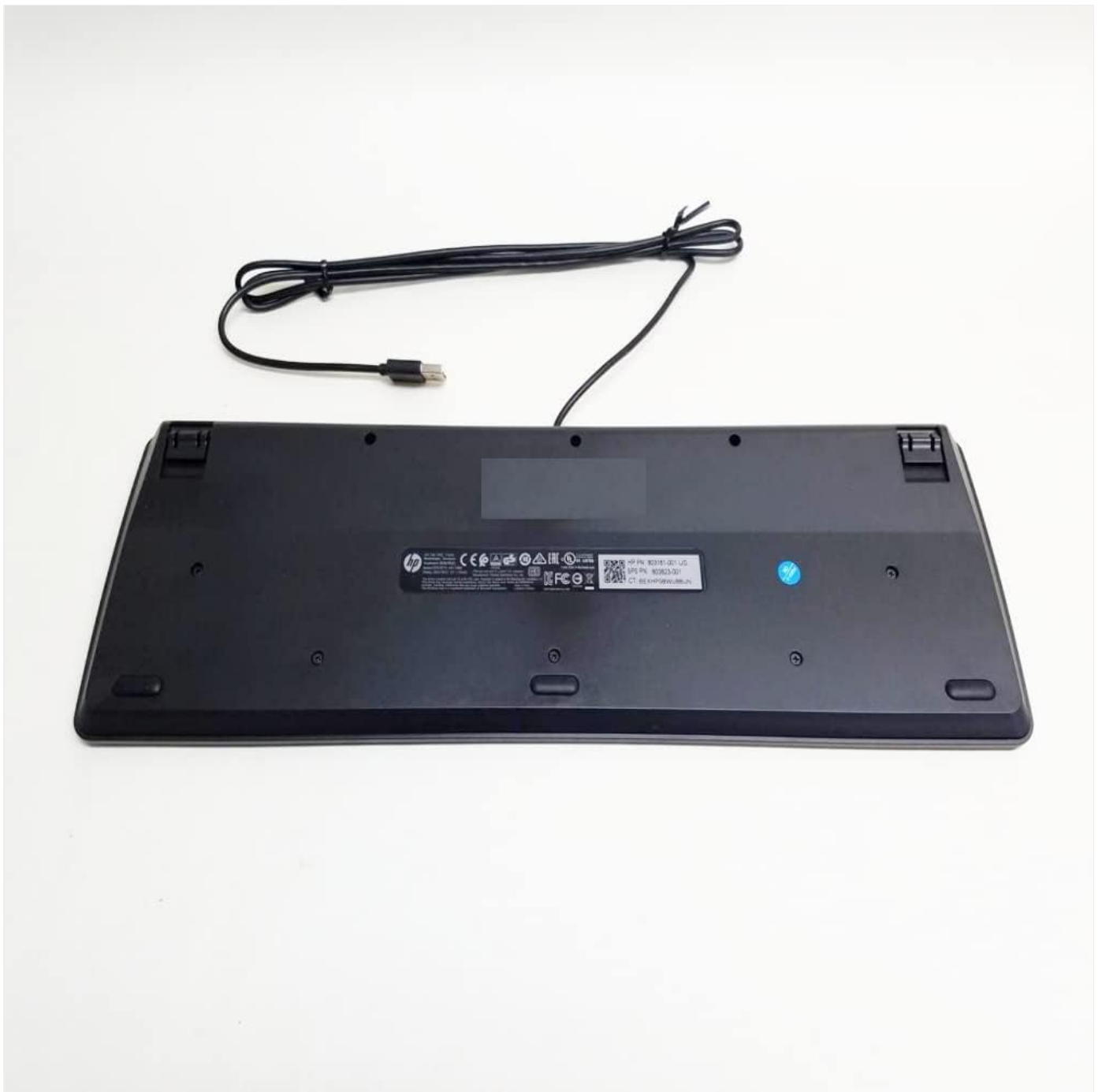
Image: The underside of the keyboard, revealing the product information label and the two adjustable flip-out feet for ergonomic positioning.
