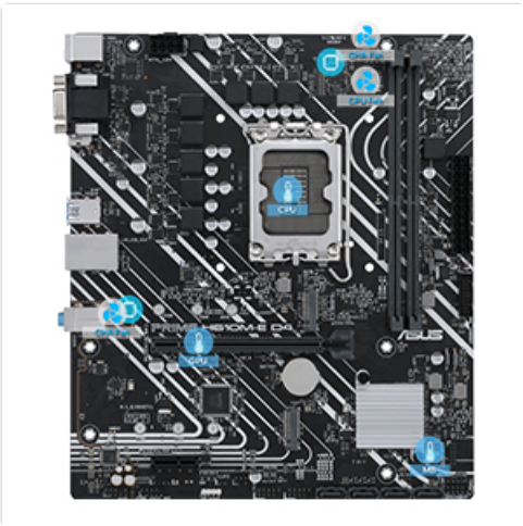
Image: Diagram indicating various cooling zones on the motherboard, including CPU, PCH, and M.2 areas, highlighting the comprehensive cooling design.
