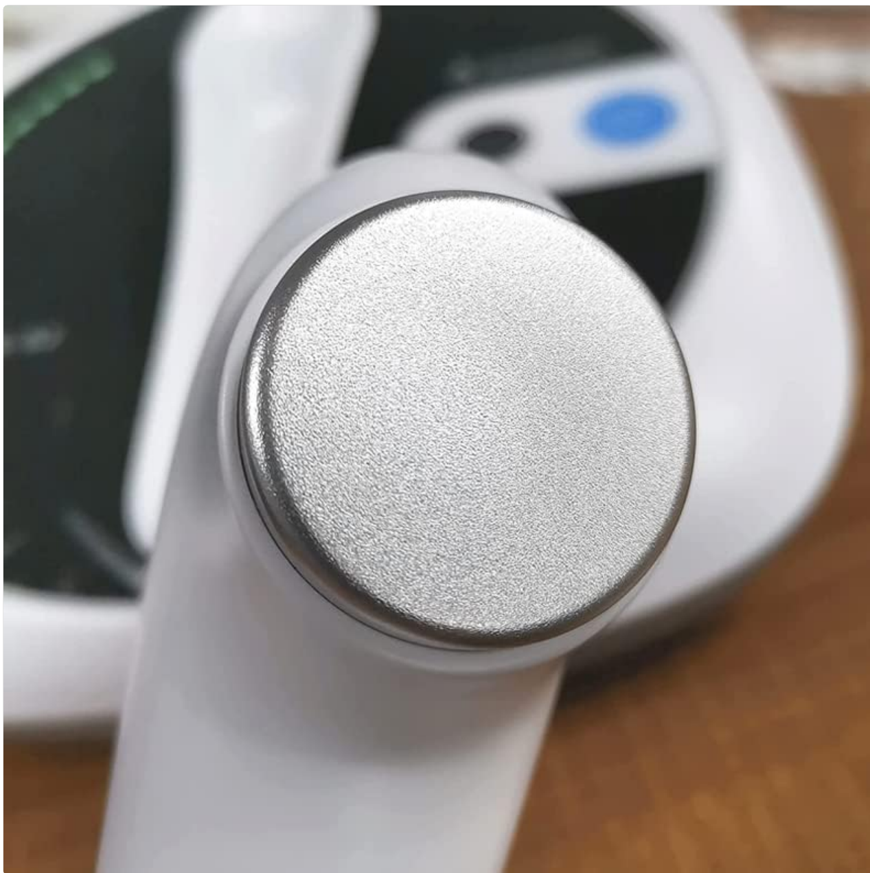
Image: A close-up view of the metal probe head, which emits the ultrasonic waves.
