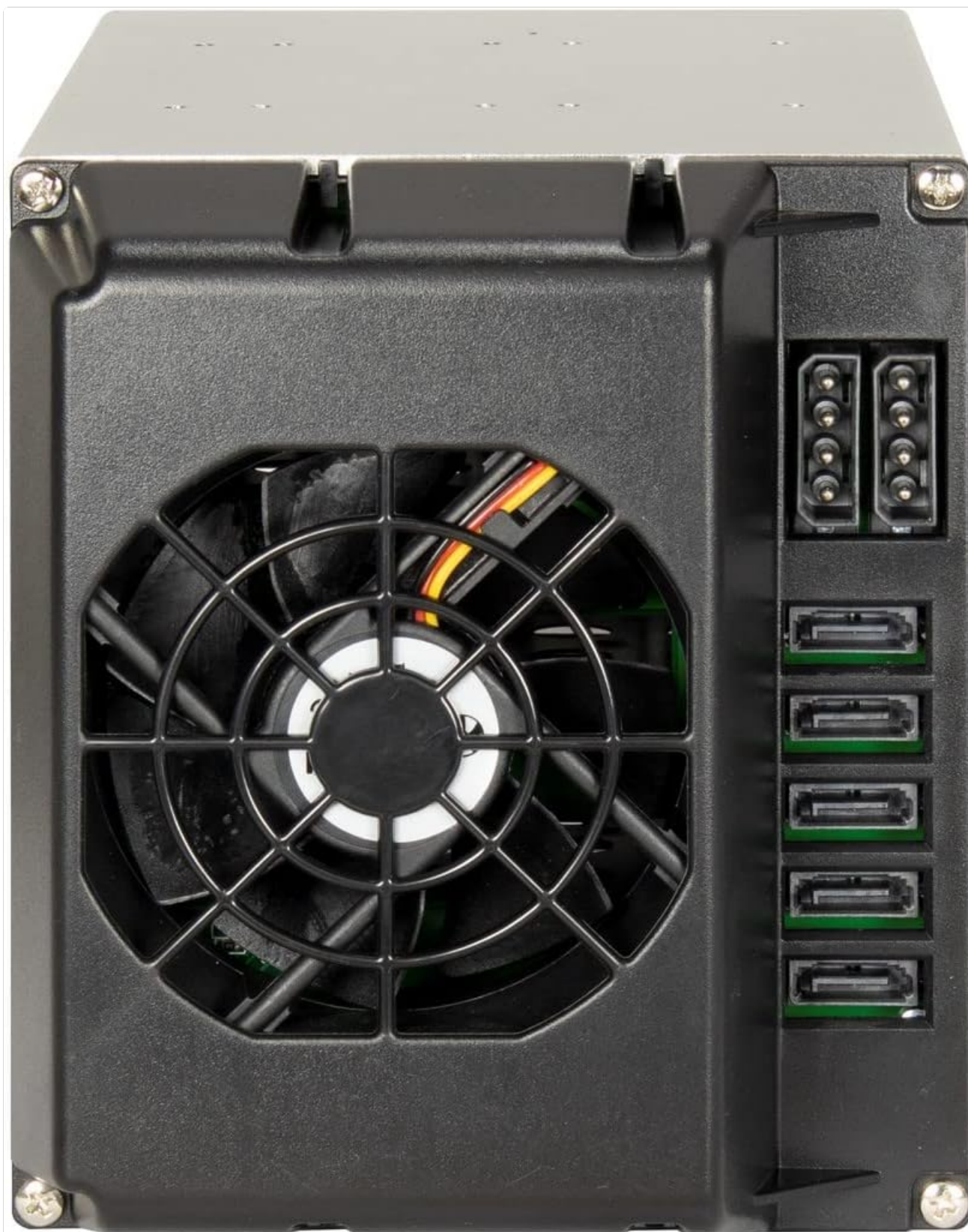
Figure 3: Rear panel of the ST-5255, illustrating the integrated 80mm cooling fan, five individual SATA data ports, and two 4-pin Molex power connectors.
