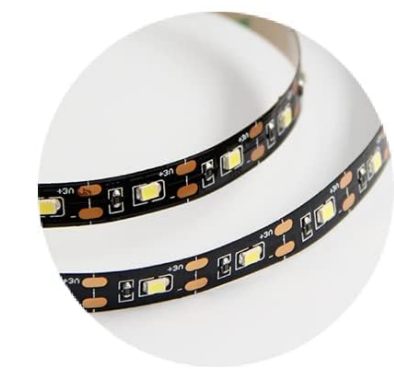
Image 4.3: LED Strip Detail. This image shows the individual LEDs on the strip and indicates where it can be safely cut to adjust length.
