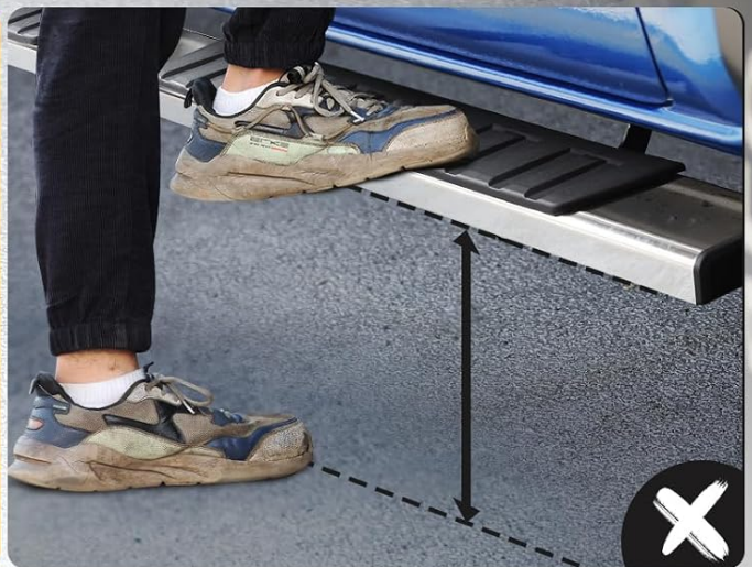
Figure 4: Illustration of the 4.7-inch drop step design for easier vehicle access.
