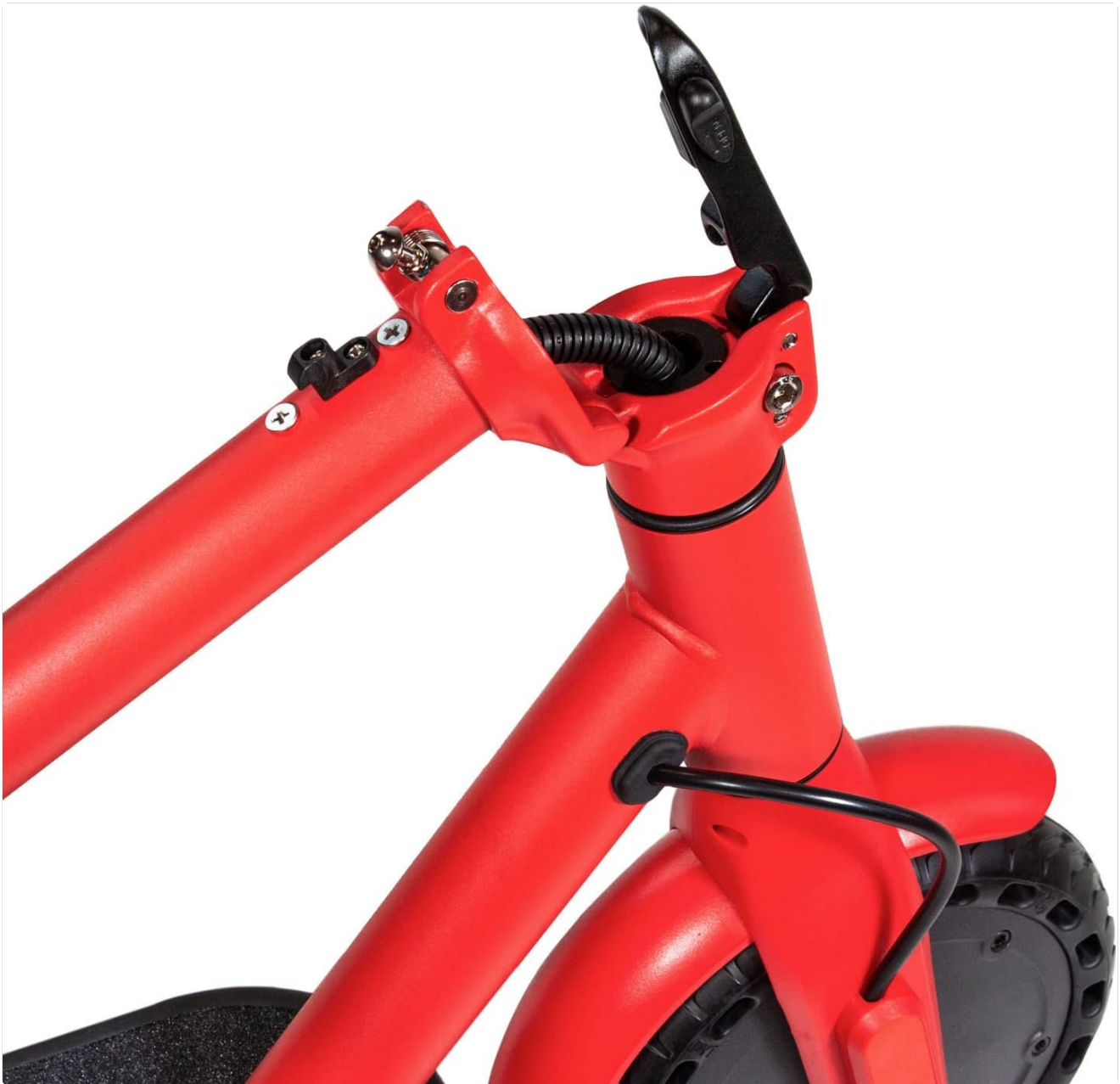
Figure 2: Detail of the scooter's folding mechanism, designed for compact storage.
