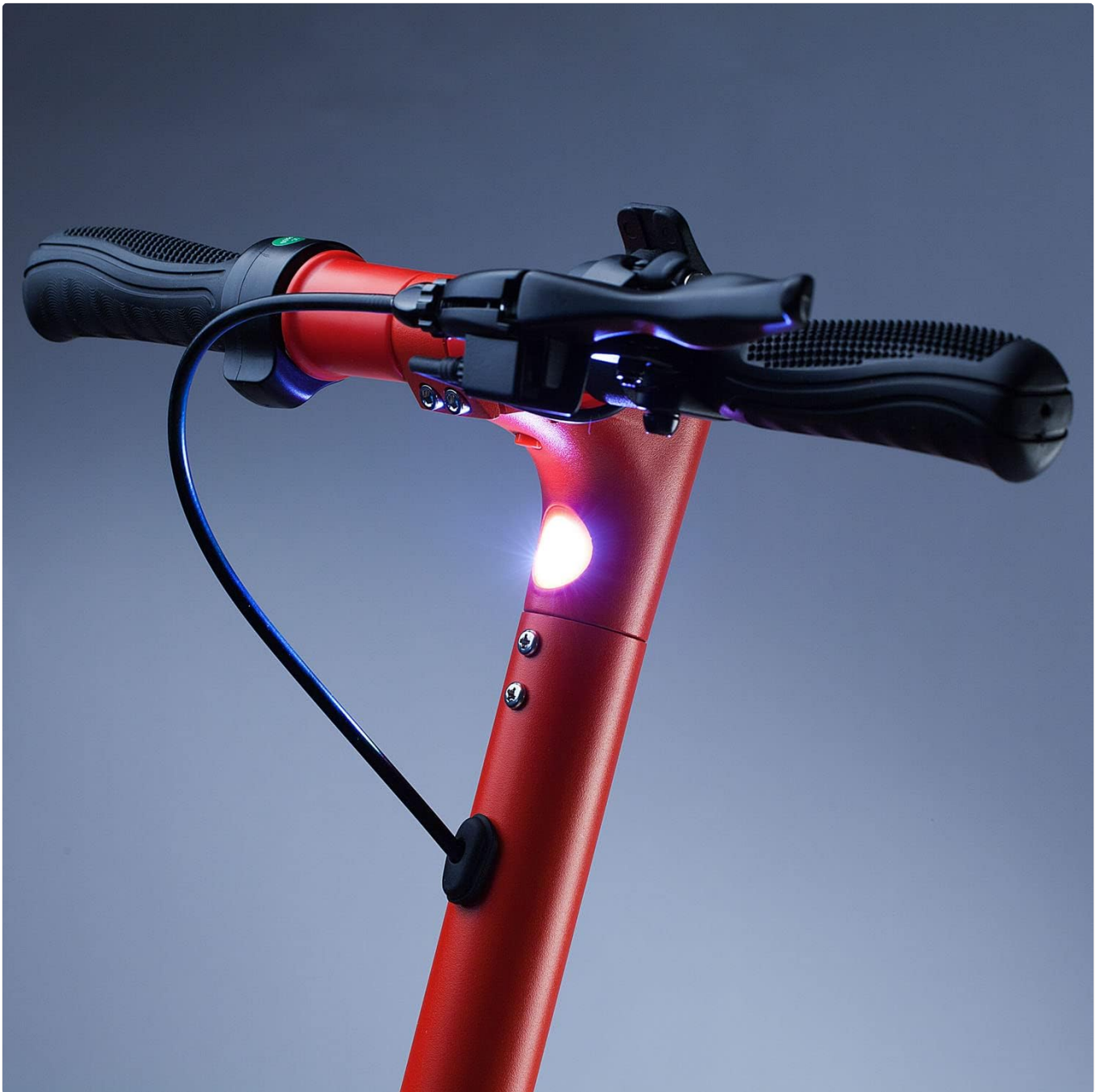
Figure 5: The scooter's integrated front light, providing illumination for night riding.
