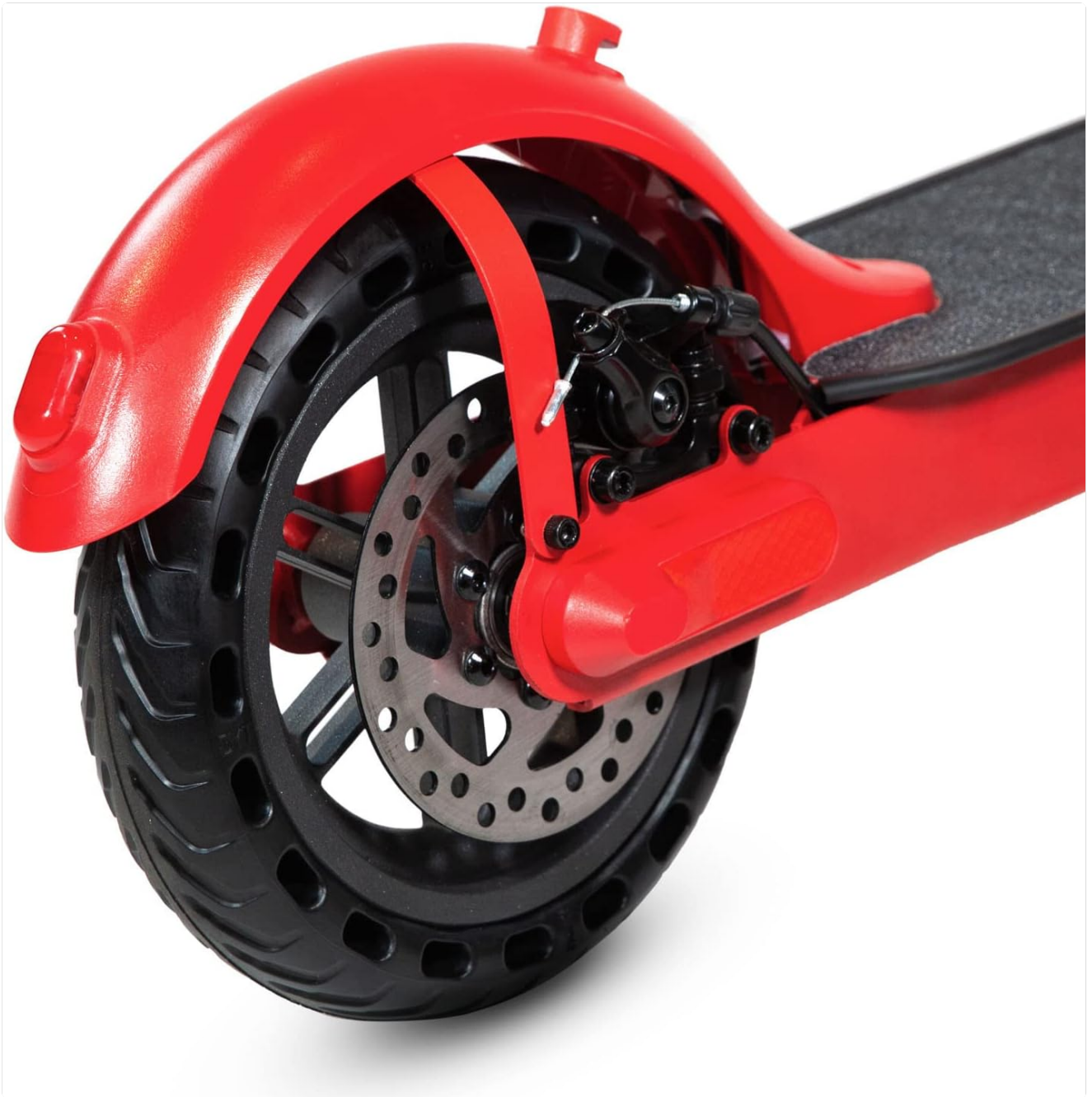
Figure 4: The rear wheel assembly, highlighting the mechanical disc brake for effective stopping power.
