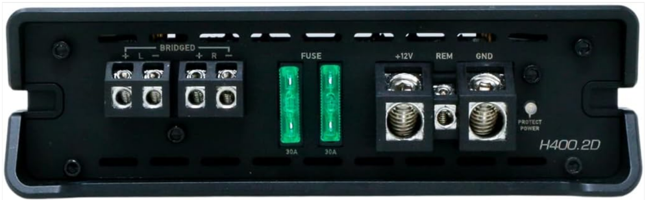
Figure 3: Rear view of the amplifier, showing the power and speaker terminal block. This section includes terminals for bridged speaker output (L+, R-), two 30A fuses, and power input terminals (+12V, REM, GND). A Protect/Power LED is also visible.
