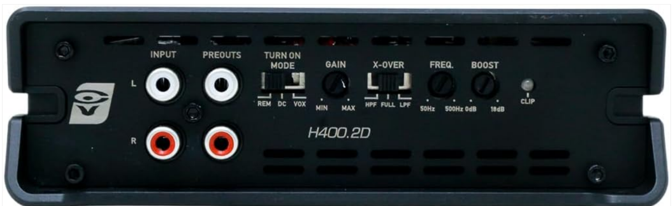
Figure 2: Front view of the amplifier, detailing the control panel. This panel includes RCA input jacks (L/R), RCA preouts, a "Turn On Mode" switch (REM, DC, VOX), Gain control, X-Over switch (HPF, FULL, LPF), Frequency (FREQ) adjustment, Boost control, and a
