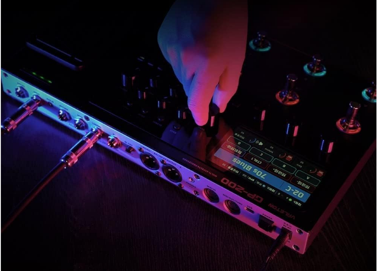
Image 4.2: A hand interacting with the Valeton GP-200's controls, demonstrating the ability to customize the effect chain with up to 11 freely movable modules working simultaneously.
