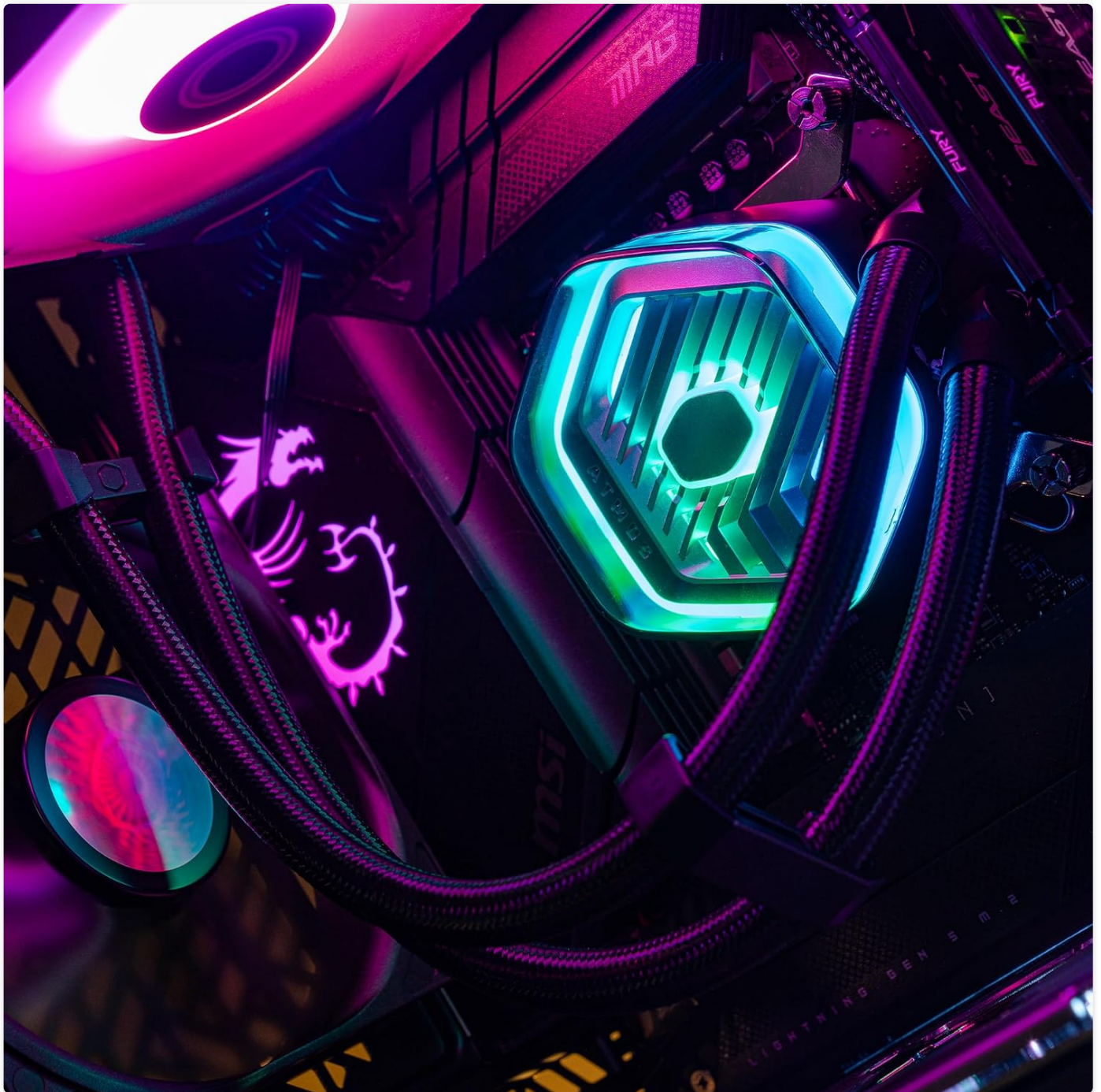
Figure 4.1: Pump Installation. This image shows the MasterLiquid Atmos 240 pump unit securely mounted on a CPU, with its vibrant ARGB lighting active, demonstrating a successful installation.
