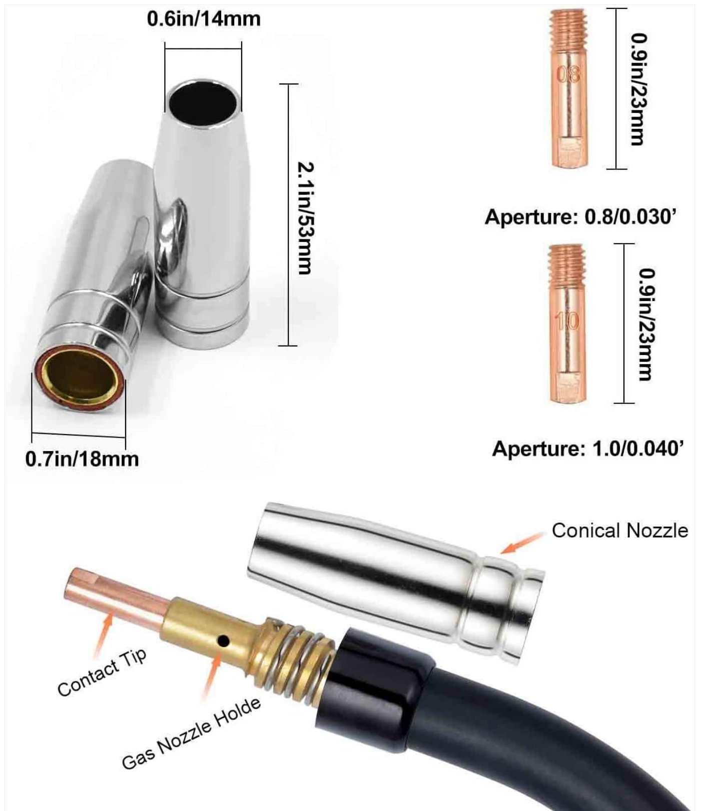
Figure 5: Detailed dimensions for the MIG welder conical nozzle and contact tips (0.8mm and 1.0mm aperture).
