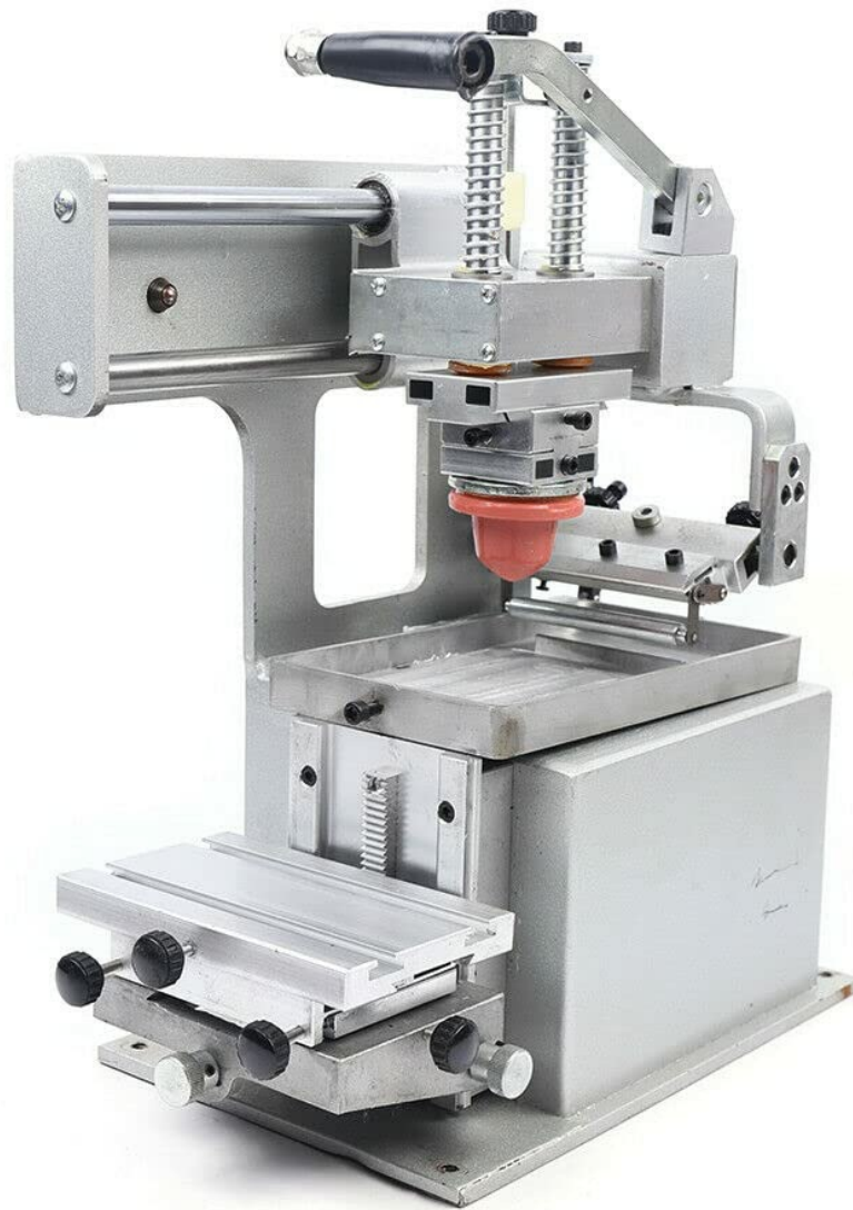
Figure 2.1: Overall view of the Gdrasuya10 Manual Pad Printer. This image displays the complete assembly of the pad printing machine, including the main body, printing arm, silicone pad, ink tray, and adjustable worktable.
