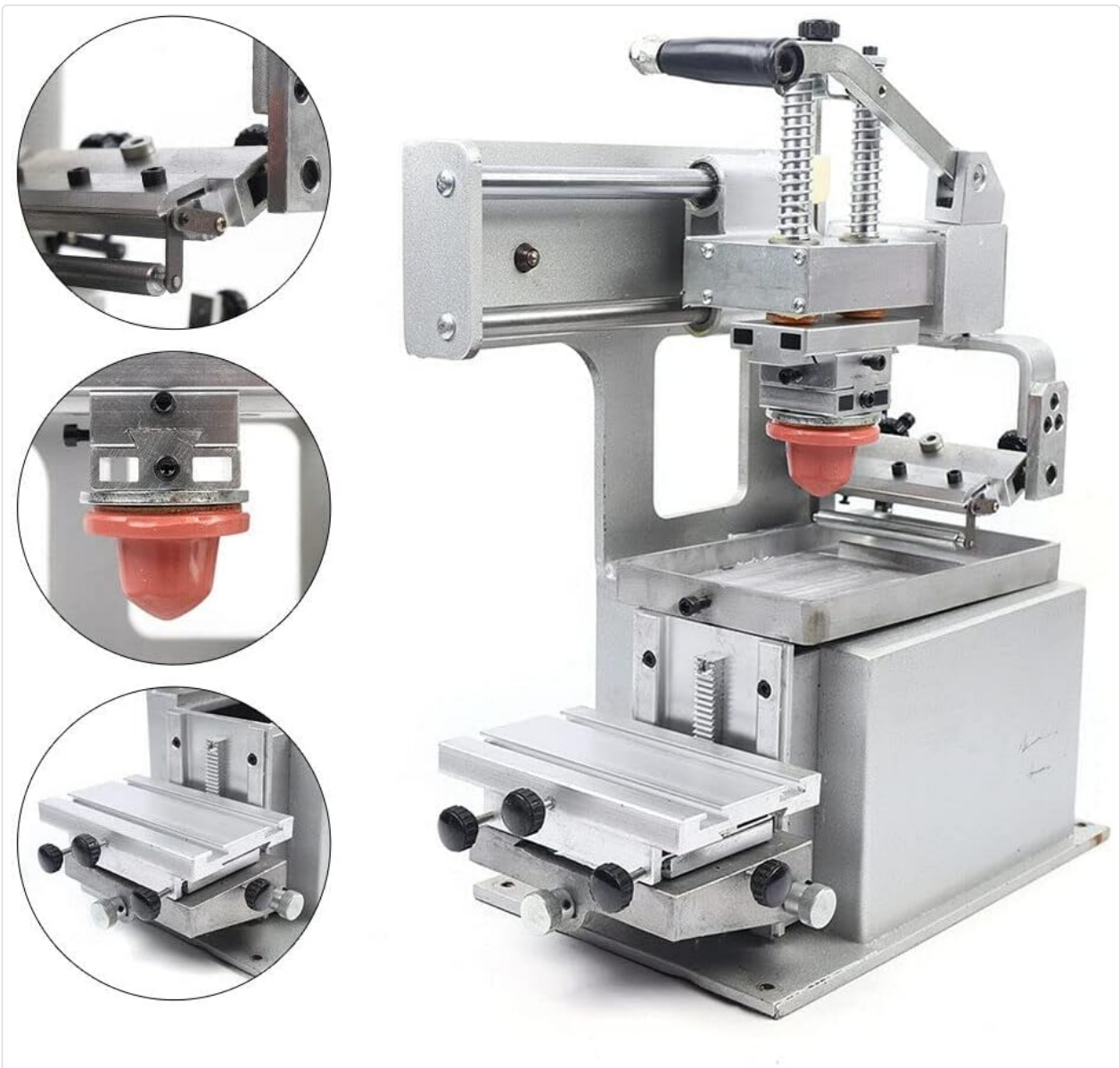
Figure 2.2: Detailed views of key components. This image shows close-ups of the red silicone printing pad, the ink tray, and the multi-directional adjustable worktable, highlighting their design and functionality.
